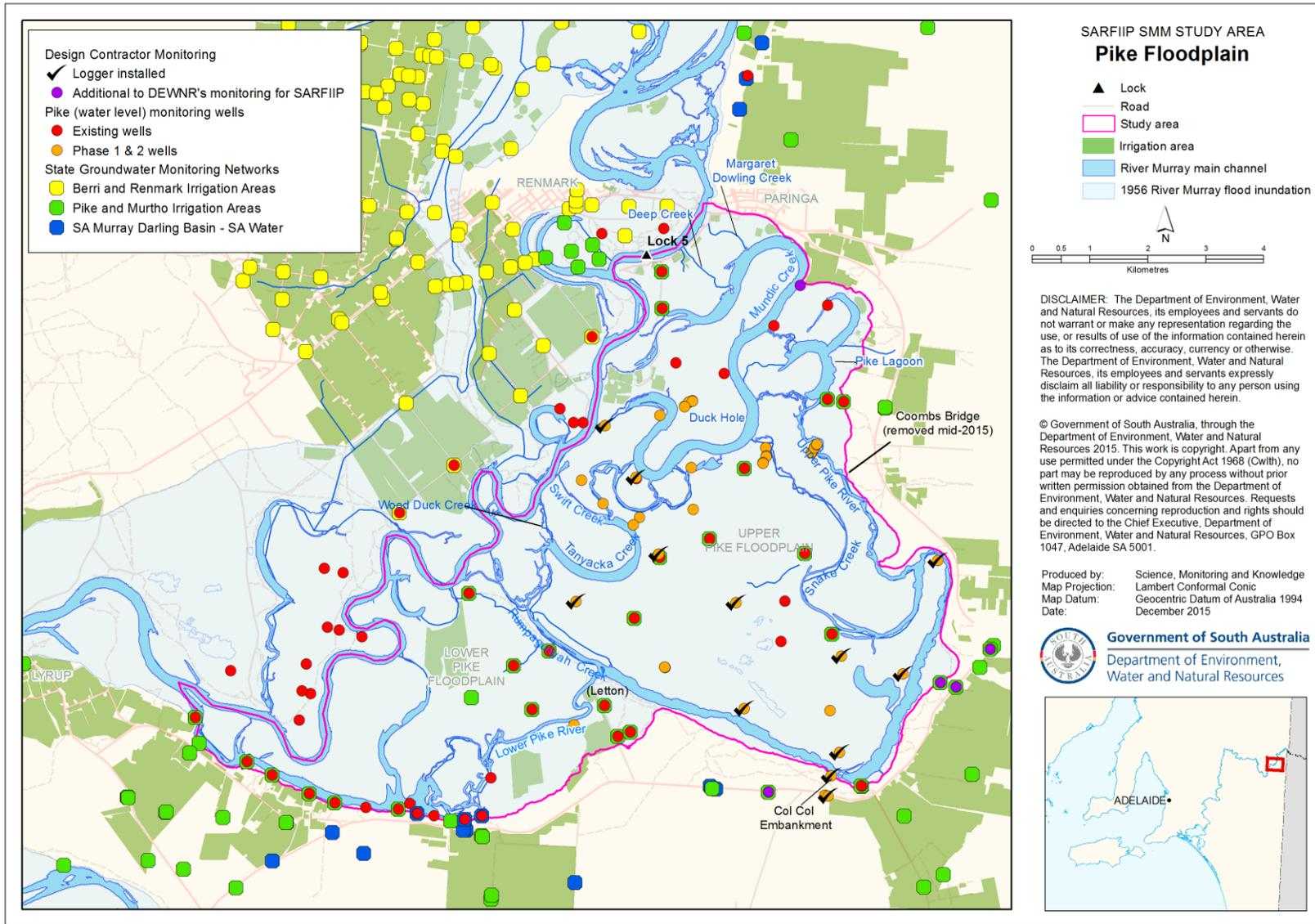
**Figure 8 Pike Floodplain 2015 groundwater level monitoring network, water level loggers and state networks**
