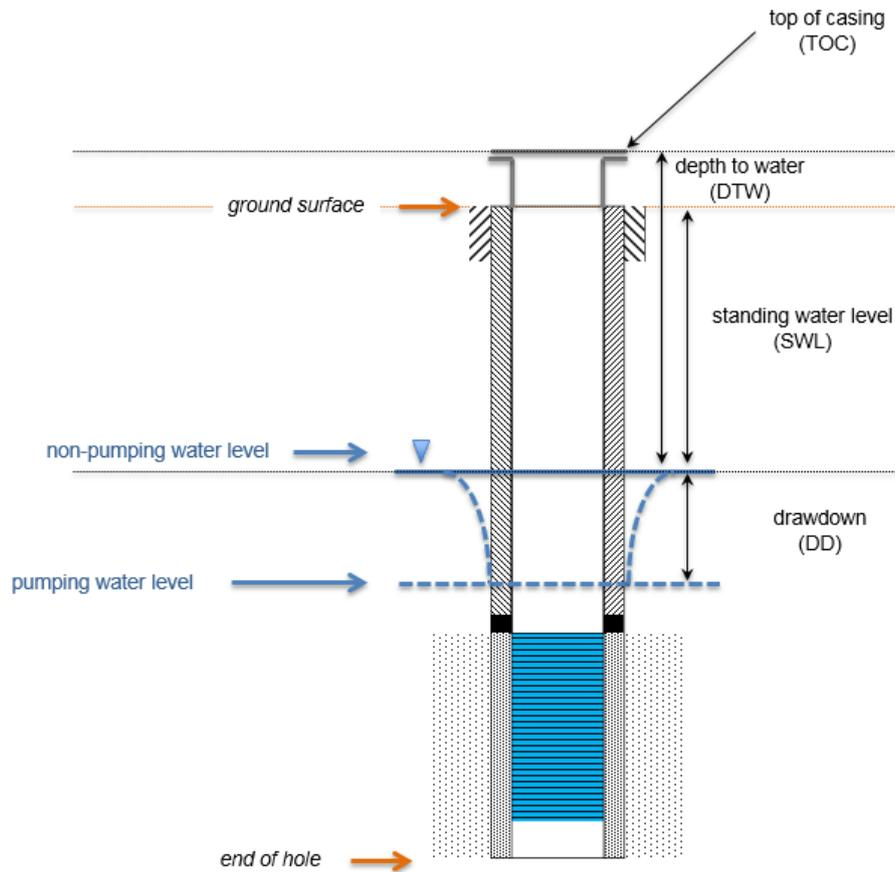
**Figure 9 Basic terms for groundwater level monitoring**
