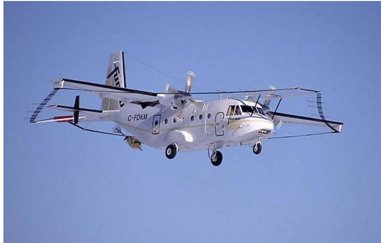
Figure 2. A fixed wing aircraft featuring the TEMPEST AEM system as used for the Jamestown and Angas-Bremer surveys (Image provided by Fugro Airborne Surveys).
