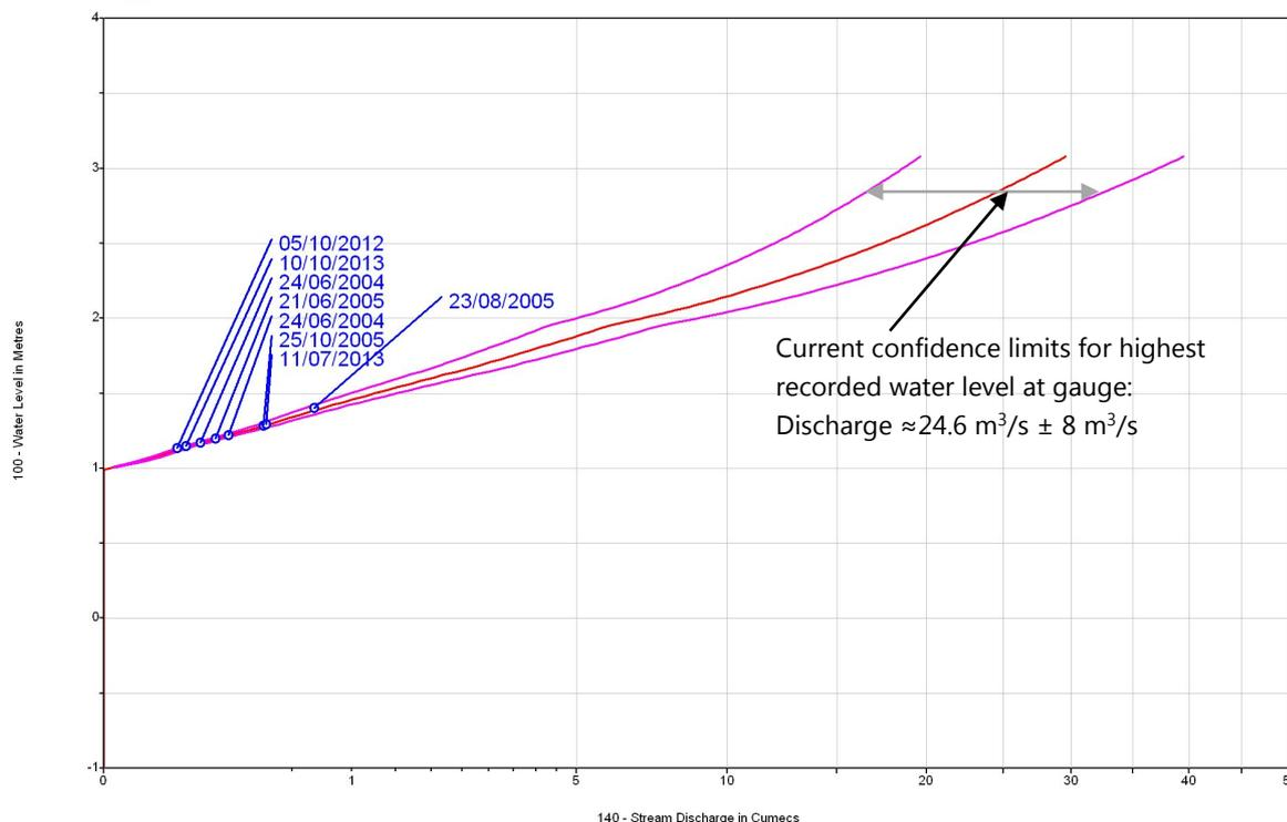
**Figure 31 Rating table (with confidence limits) used to describe flows passing the Timber Creek streamflow gauge (site A5131002) as at May 2014, with individual gaugings shown**
