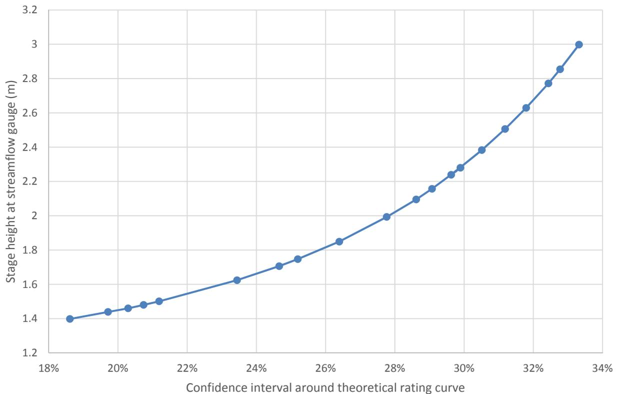
**Figure 33 Variation in confidence interval around theoretical rating curve for the Timber Creek streamflow gauge**
