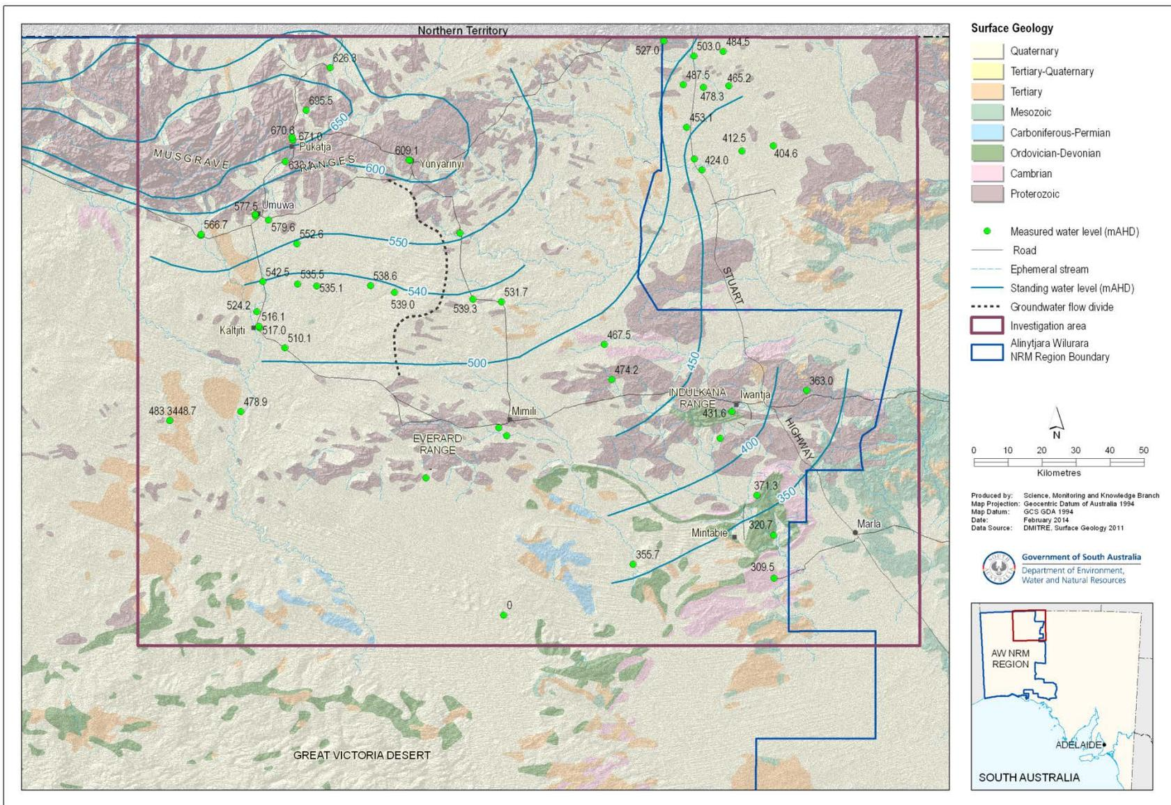
Figure 8. Watertable contours for the unconfined aquifer
