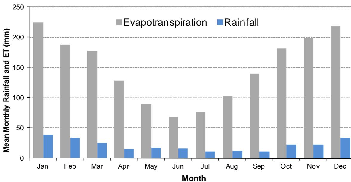
**Figure 4. Measured mean monthly rainfall and estimated potential evapotranspiration (FAO56) at Pukatja**
