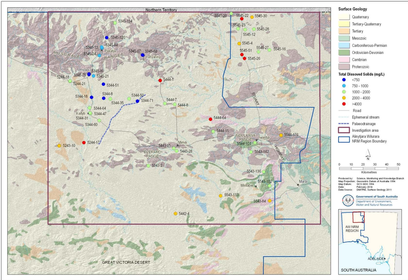
Figure 9. Groundwater salinity (TDS) in the investigation area with wells identified by their unit number
