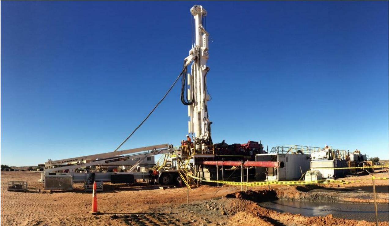
**Figure 4. Rod loading, blooey line and mud system used for Mulka Bore No. 2**
