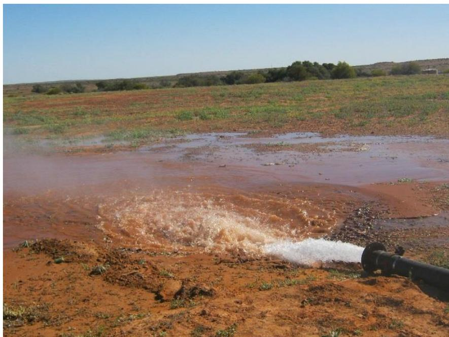
**Figure 10. Artesian flow of 36 L/s from Mulka Bore No. 2 during flow test on 4 August 2016**
