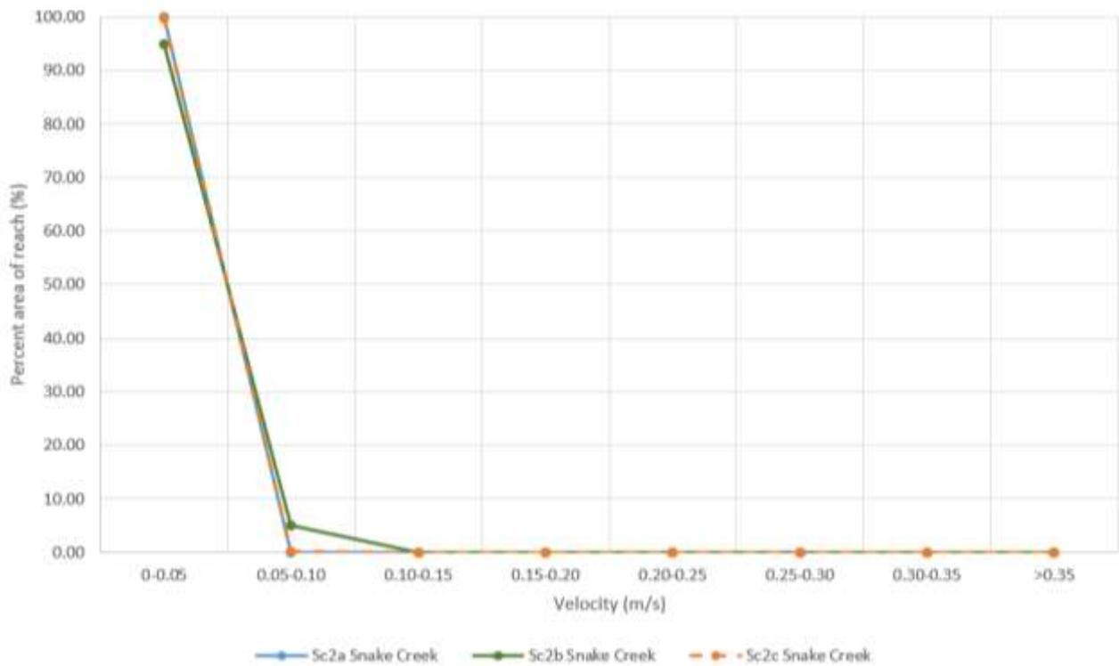
**Figure 4.9 Velocity distribution by percent of reach in Snake Creek for Scenario 2 simulations (refer to Figure 2.1 for location)**
