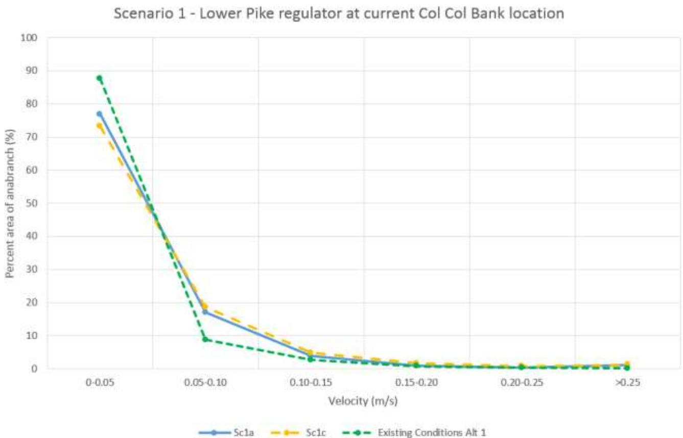
**Figure A.1 Velocity profiles by percent of anabranch for Scenarios 1a and c (i.e. Pike regulator at current Col Col location) compared to existing floodplain conditions at equivalent flow regime**
