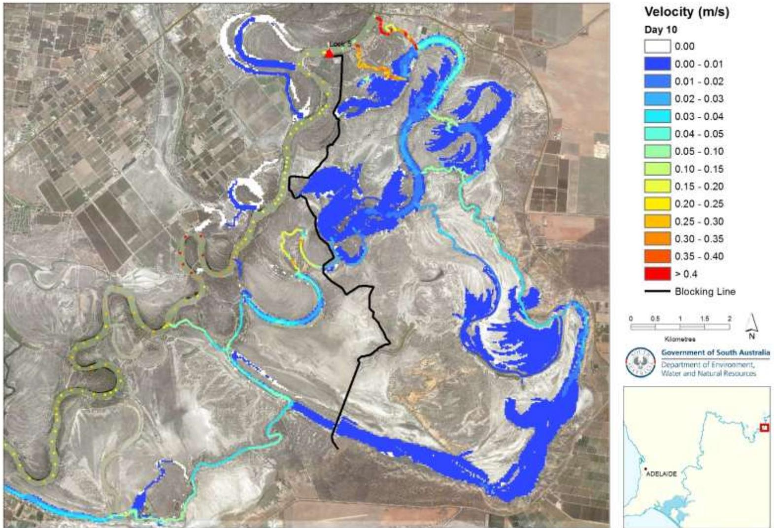
**Figure 9.14 Velocity distribution at Day 10 (water level at Pike Regulator 15.59 m AHD) of managed inundation under Alternative 2 blocking alignment**
