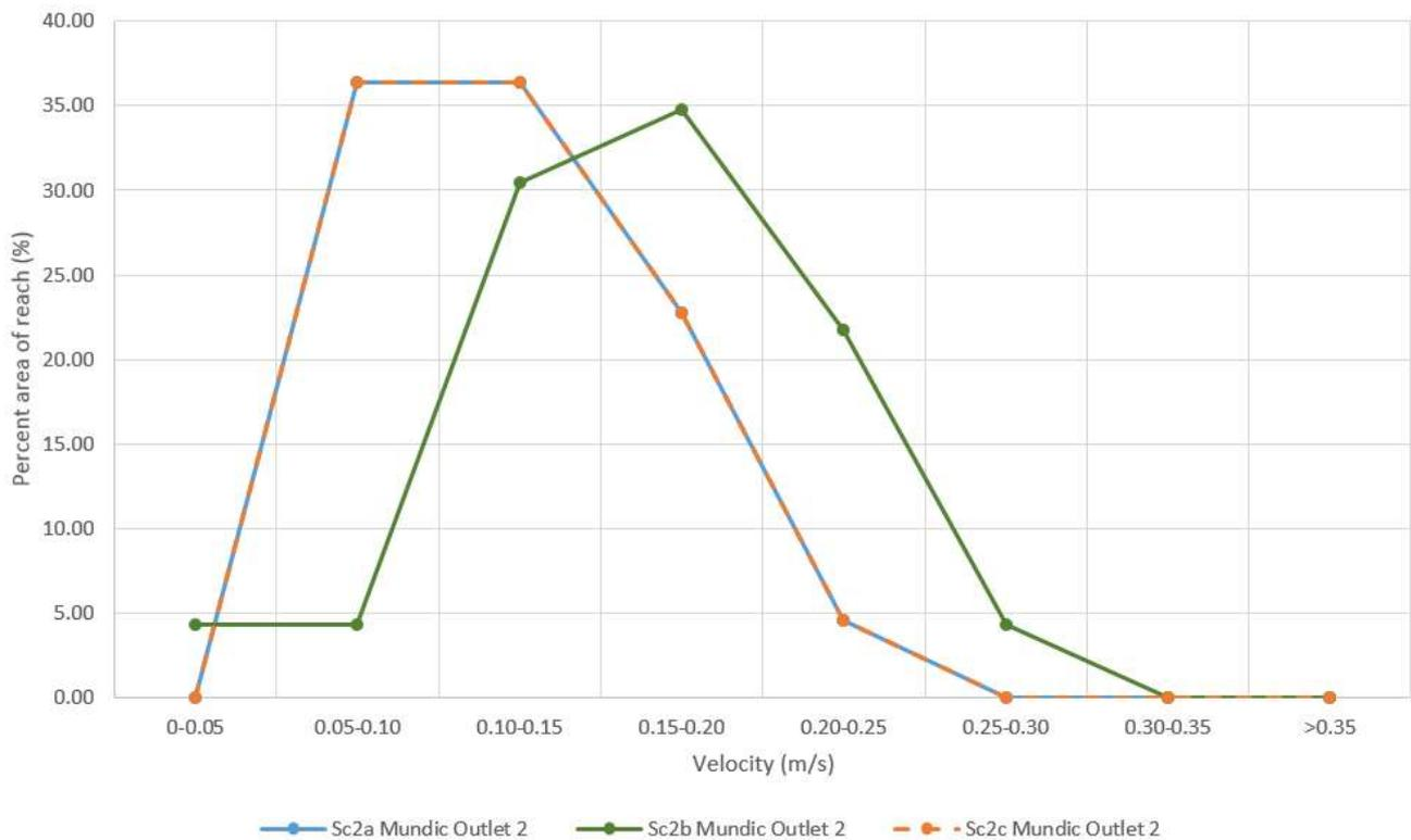
**Figure 4.8 Velocity distribution by percent of reach in Mundic Creek Southern Outlet for Scenario 2 simulations (refer to Figure 2.1 for location)**
