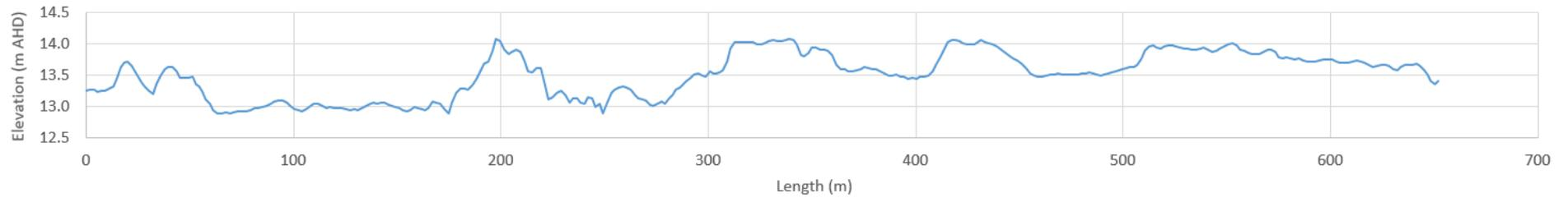
**Figure 10.2 Long section of Letton’s flood runner inlet showing approximate minimum levels along the flow path from River Murray to Lower Pike River**
