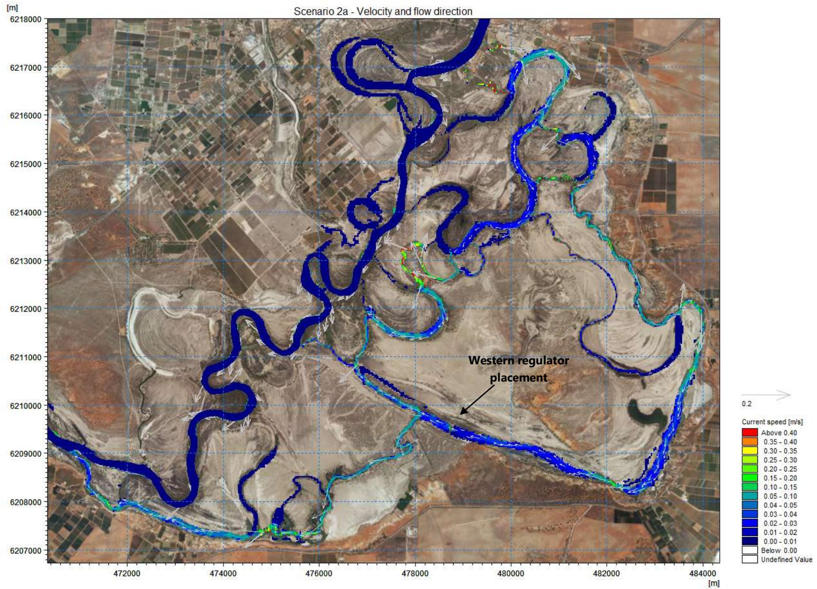
**Figure 4.2 Velocity and flow direction for an inflow of 800 ML/d and Tanyaca flow of 400 ML/d (Scenario 2a)**
