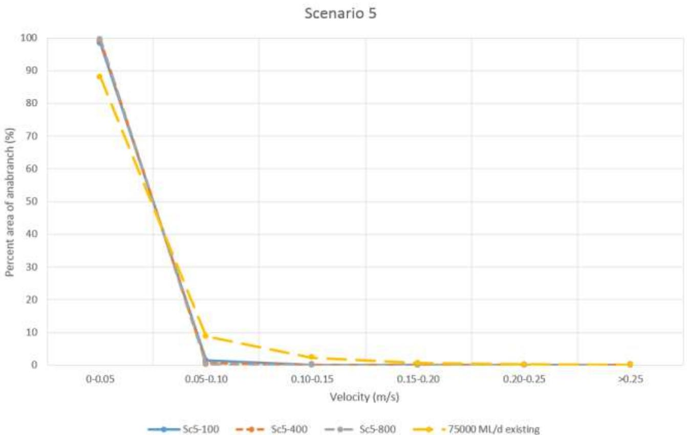
**Figure A.6 Velocity profiles by percent of anabranch for Scenario 5 (Tanyaca flow at 100, 400 and 800 ML/d) compared to existing floodplain conditions with an equivalent flow regime (i.e. 75 000 ML/d flow upstream of Lock 5)**
