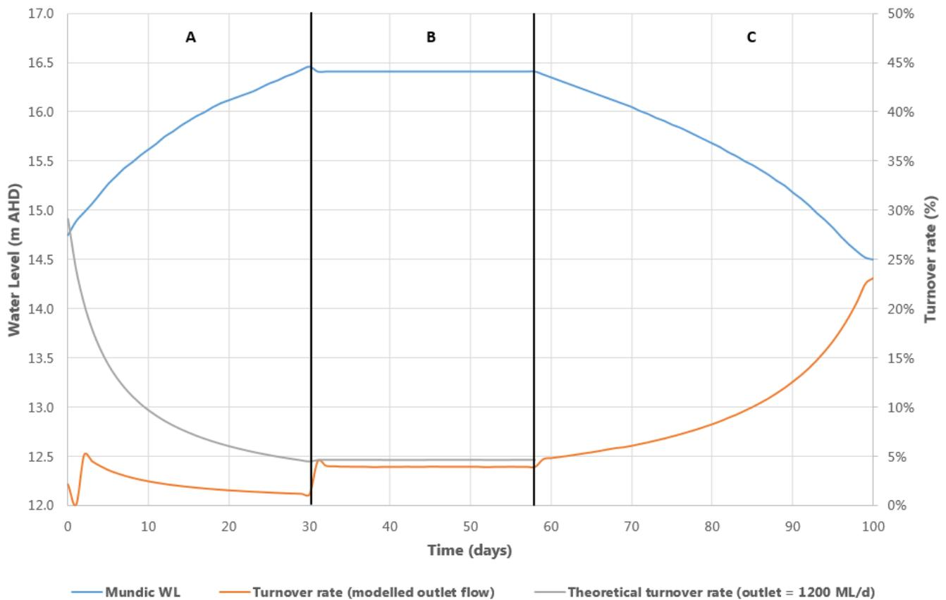
**Figure 9.3 Modelled turnover rate (based on modelled outlet flow) and theoretical turnover rate (outlet flow based on maximum inlet flow of 1200 ML/d), during managed inundation event, with reference to Mundic Creek water level. Various phases of operation indicated: A – Filling phase; B – Holding phase; and C – Draining phase.**
