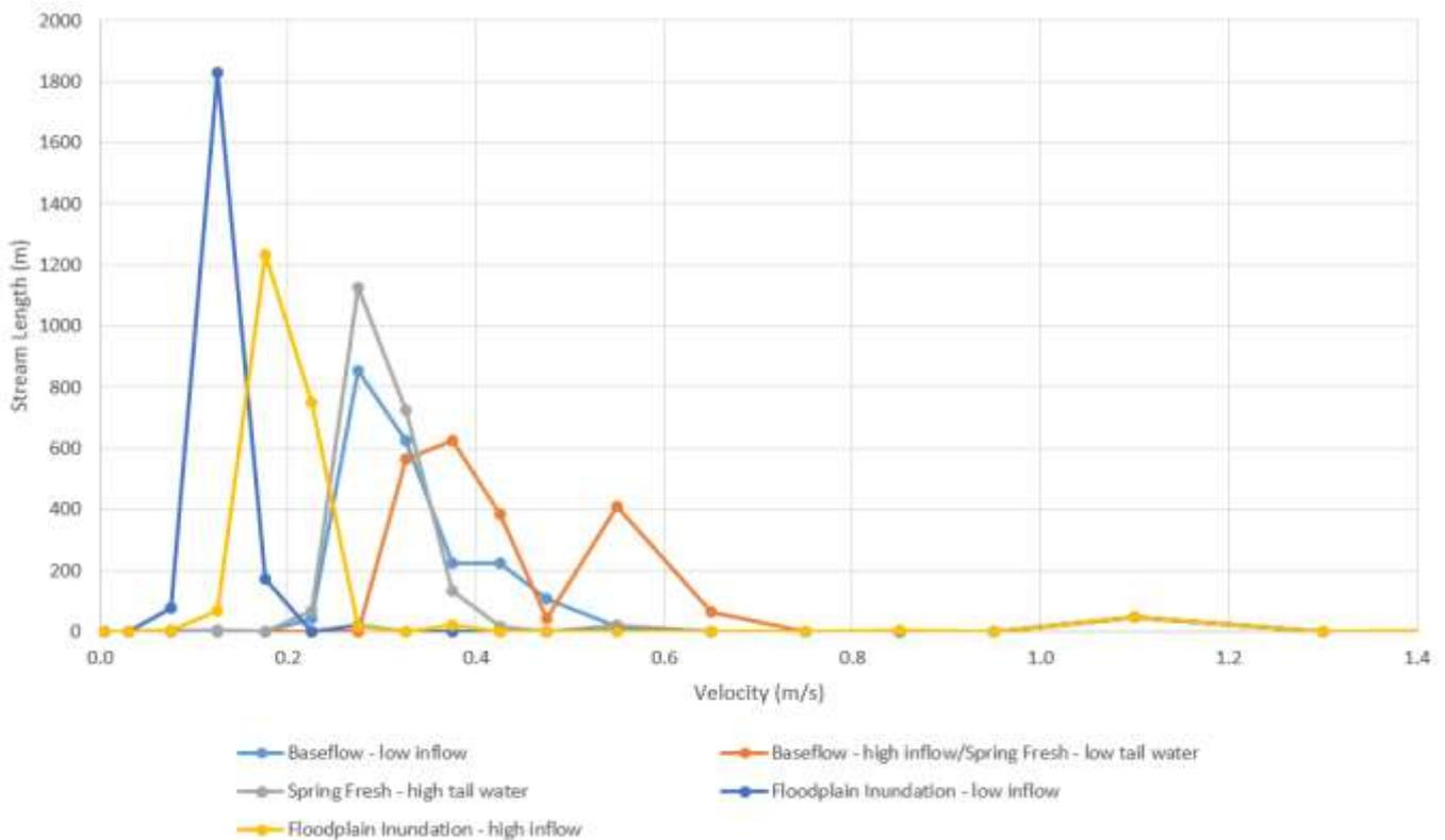
**Figure 11.2 Deep Creek velocity profiles by stream length, from Table 11.2**
