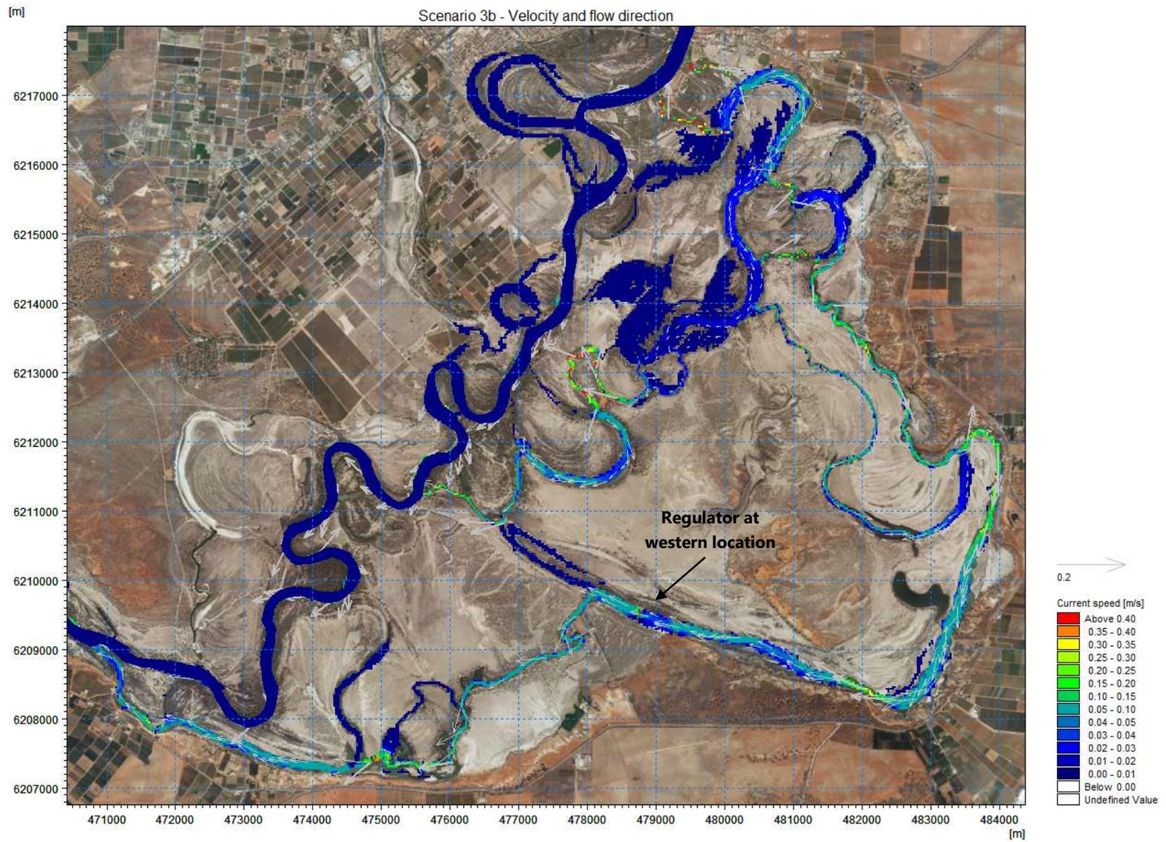
**Figure 5.4 Velocity and flow direction for an inflow of 1200 ML/d and minor regulators on Mundic Creek outlets passing 800 ML/d (Scenario 3b)**
