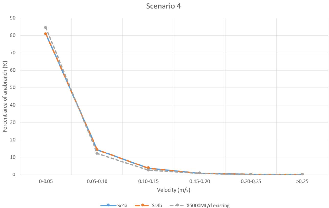
**Figure A.5 Velocity profiles by percent of anabranch for Scenarios 4a and b compared to existing floodplain conditions with an equivalent flow regime (i.e. 85 000 ML/d flow upstream of Lock 5)**
