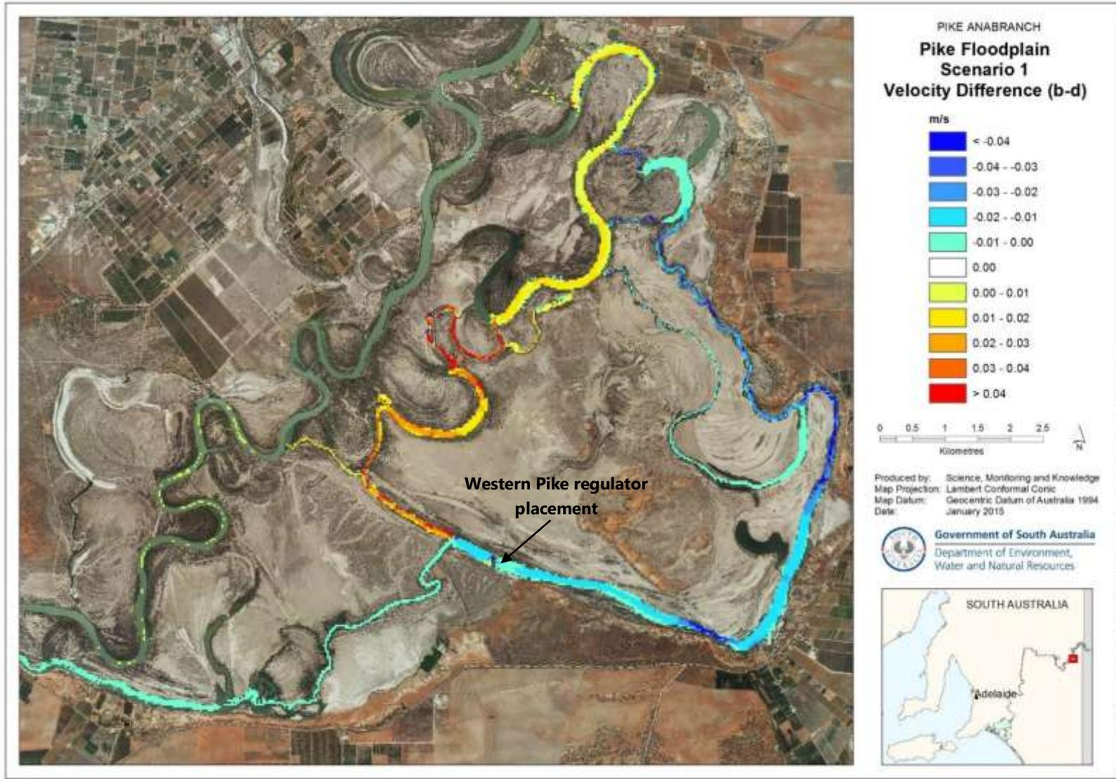
**Figure 3.8 Velocity difference over entire floodplain with western Pike regulator alternative between Tanyaca flows of 600 and 400 ML/d, respectively**
