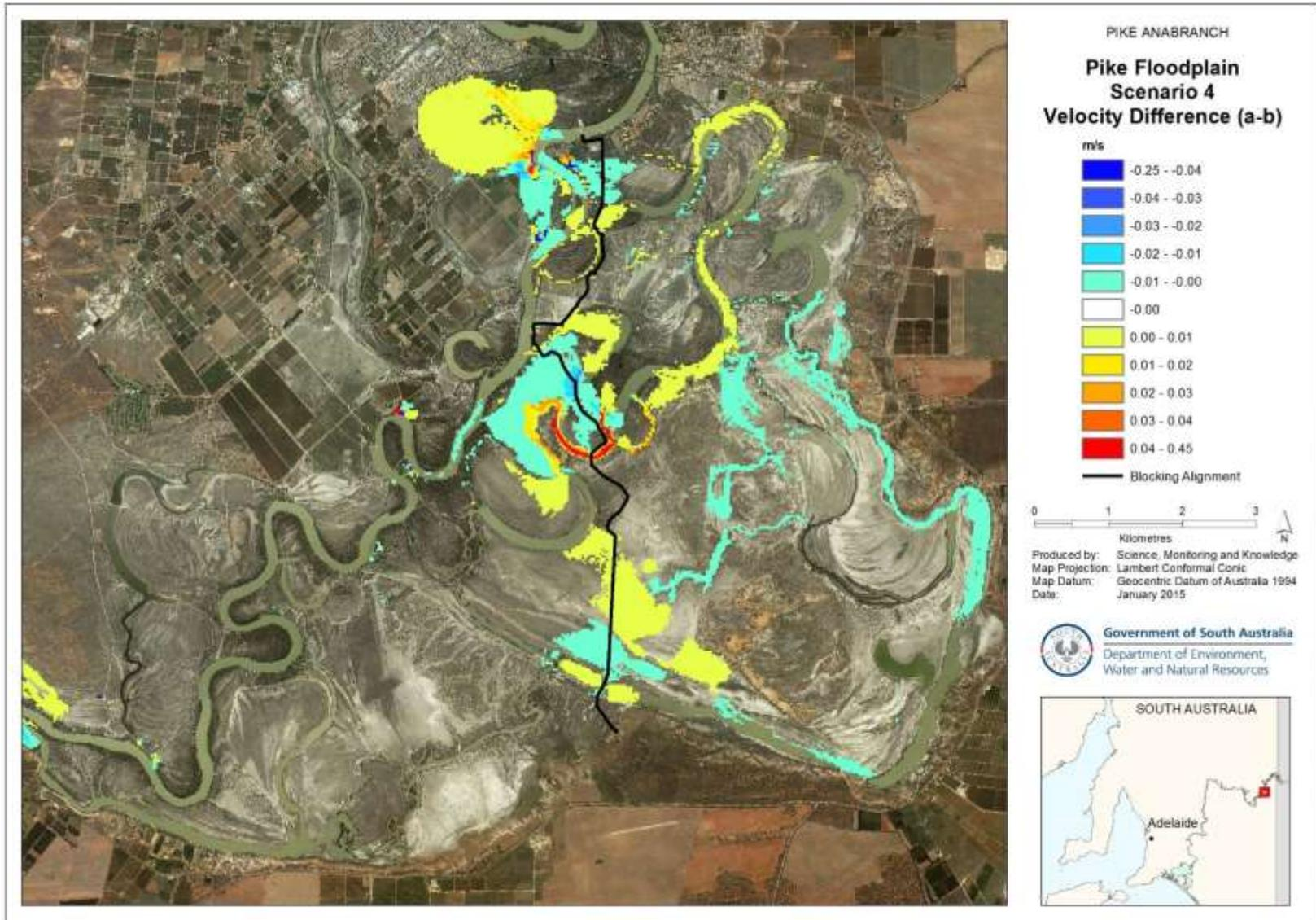
**Figure 6.3 Velocity difference encountered at a River Murray flow of 90 000 ML/d between 100% and 50% concept design regulator sizes**
