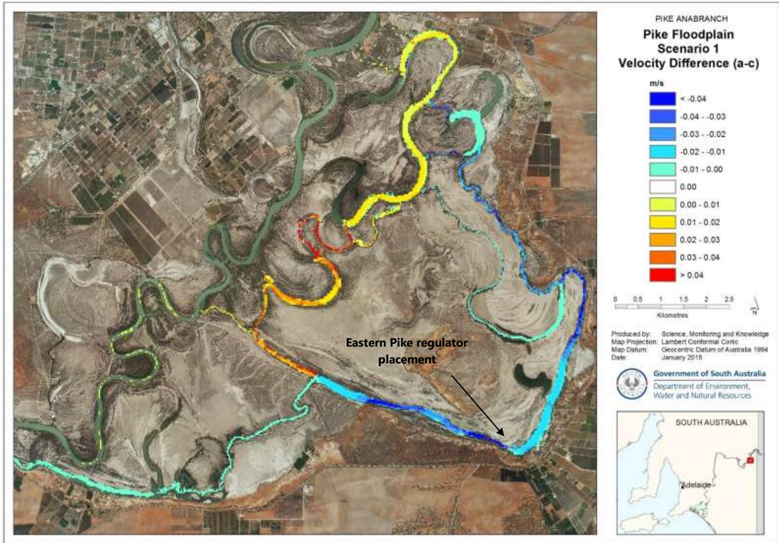
**Figure 3.7 Velocity difference over entire floodplain with eastern Pike regulator alternative between Tanyaca flows of 600 and 400 ML/d, respectively**
