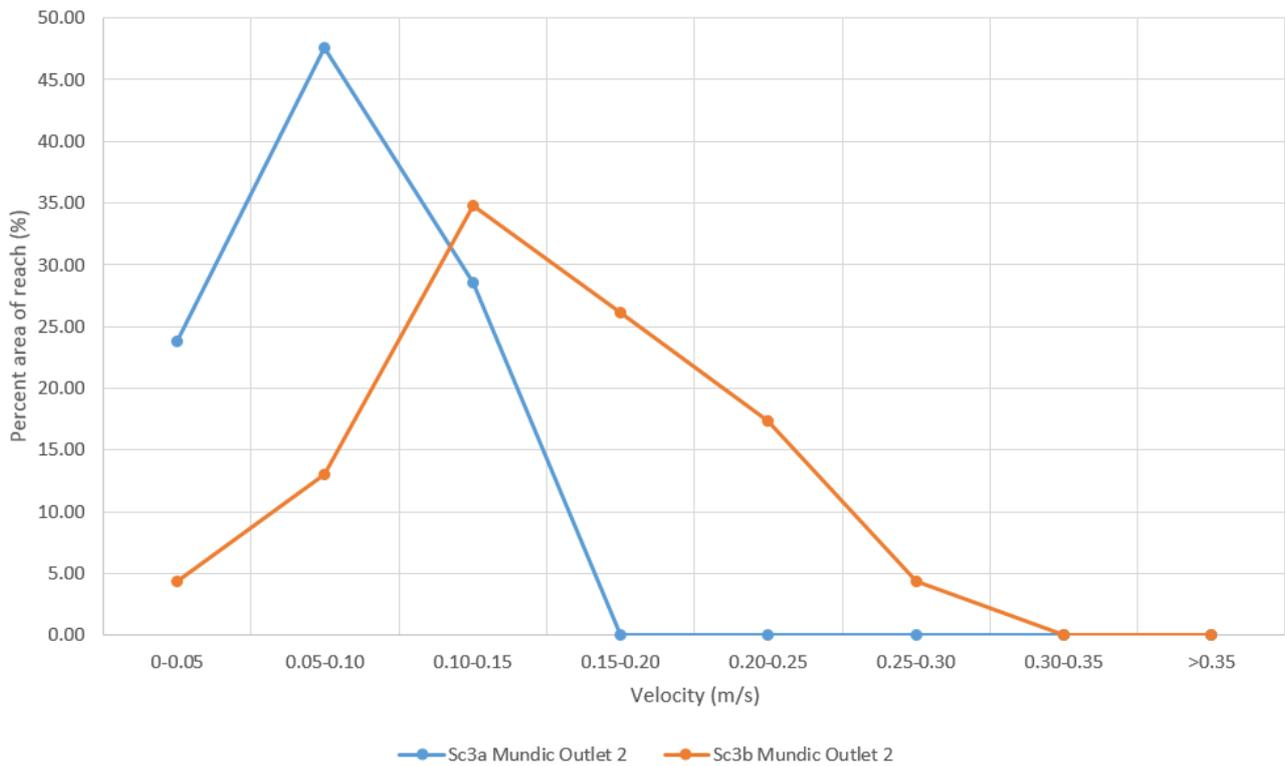
**Figure 5.6 Velocity distribution by percent of reach in Mundic Creek Southern Outlet for Scenario 3 simulations (refer to Figure 2.1 for location).**
