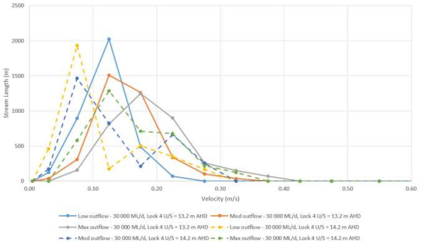
**Figure 11.6** Tanyaca Creek velocity profiles by stream length, river flow 30 000 ML/d, from Table 11.6
