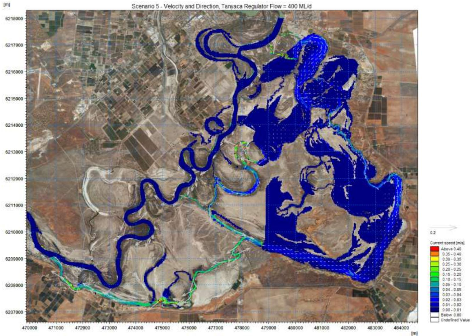
**Figure 7.5 Velocity distribution and flow direction at an inundation level of 16.4 m AHD with alternative Pike River environmental regulator placement and a flow of 400 ML/d through Tanyaca Creek**
