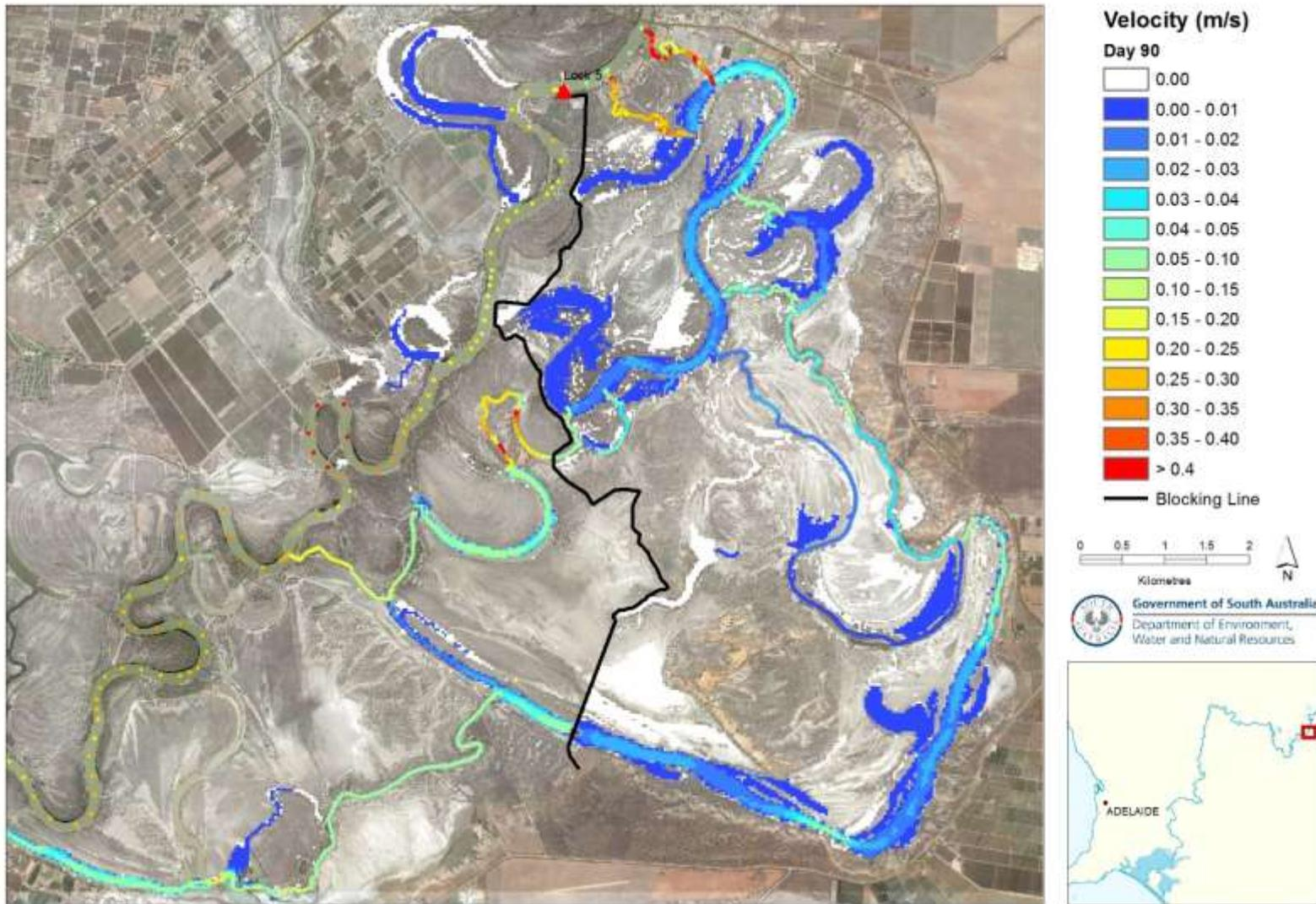
**Figure 9.22 Velocity distribution at Day 90 (water level at Pike Regulator 15.12 m AHD) of managed inundation under Alternative 2 blocking alignment**
