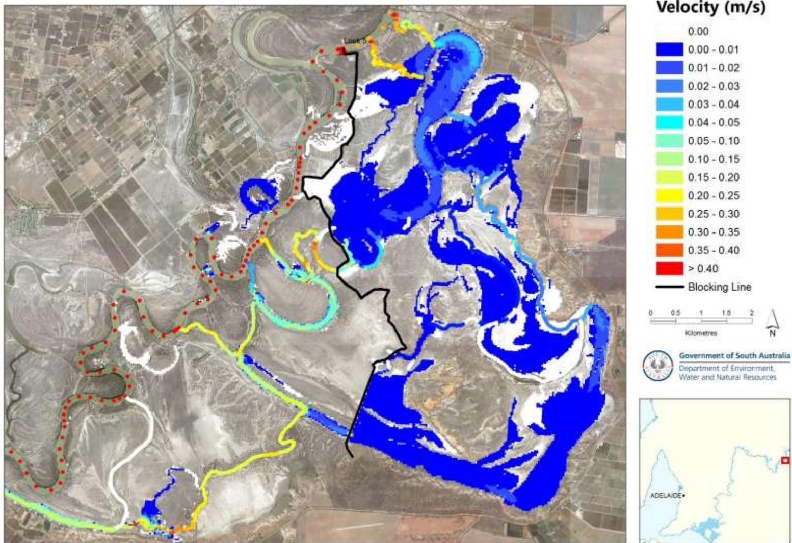
**Figure 10.6 Velocity distribution in Pike Floodplain at flow upstream of Lock 5 at 30 000 ML/d and typical Lock 4 weir pool level at 13.2 m AHD under managed inundation operating conditions**
