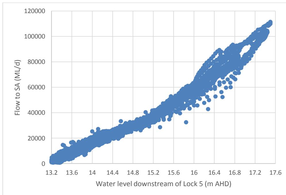
**Figure 7.1 Flow to South Australia versus water level downstream of Lock 5**
