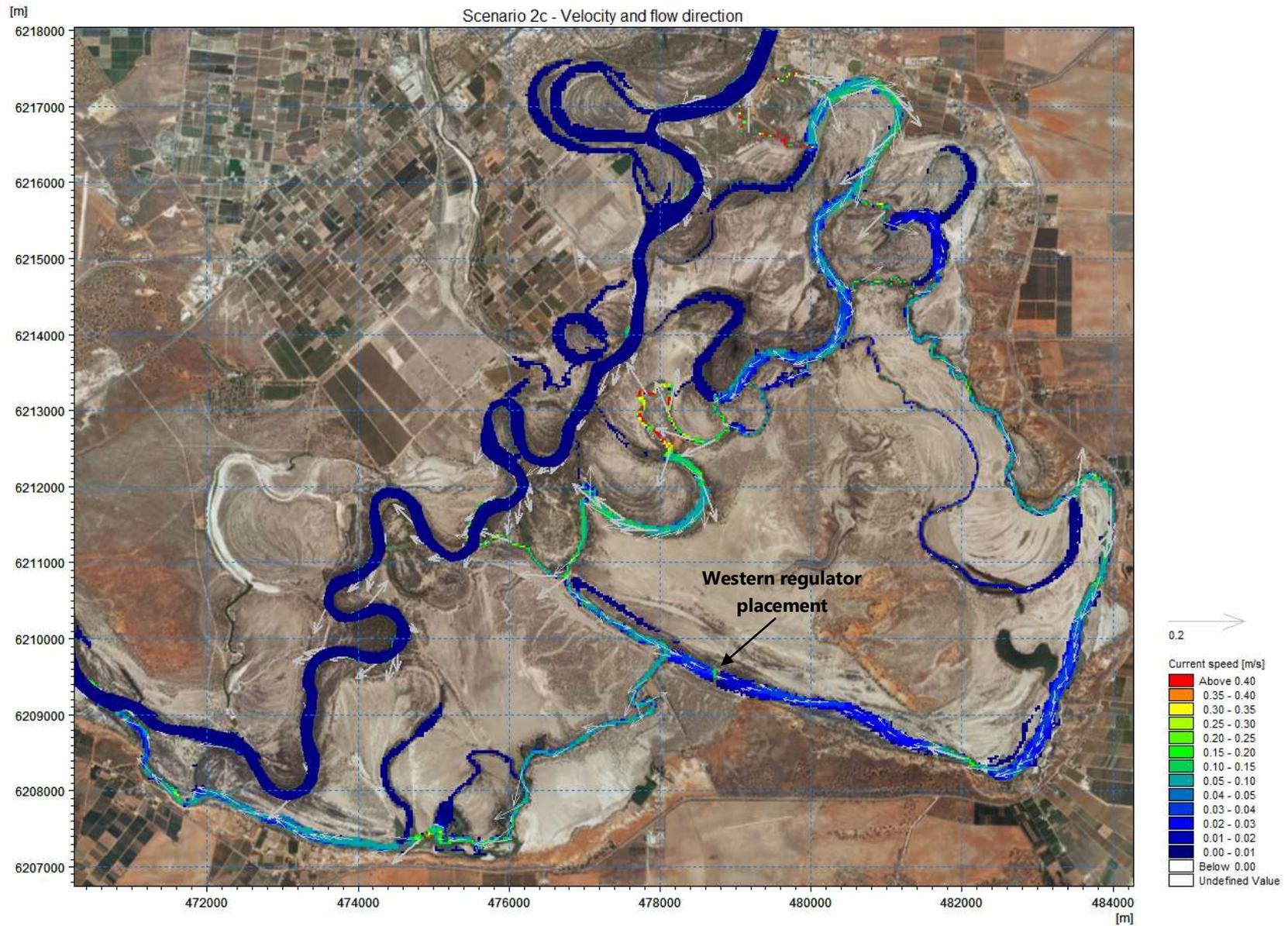
**Figure 4.6 Velocity and flow direction for an inflow of 1200 ML/d and Tanyaca flow of 800 ML/d (Scenario 2c)**
