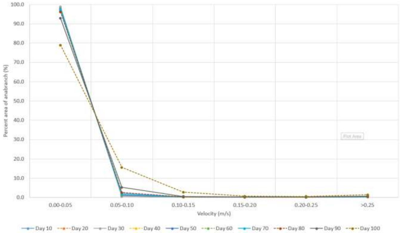
**Figure A.8 Velocity profiles by percent of anabranch for Scenario 7, shown in 10-day increments over the duration of the modelled managed inundation event**
