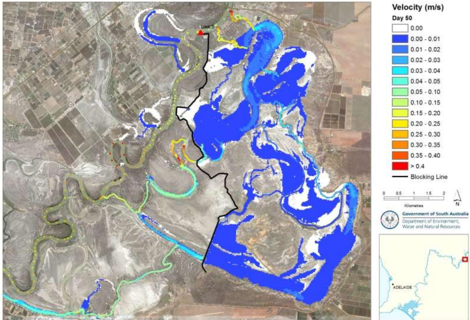
**Figure 9.18 Velocity distribution at Day 50 (water level at Pike Regulator 16.40 m AHD) of managed inundation under Alternative 2 blocking alignment**
