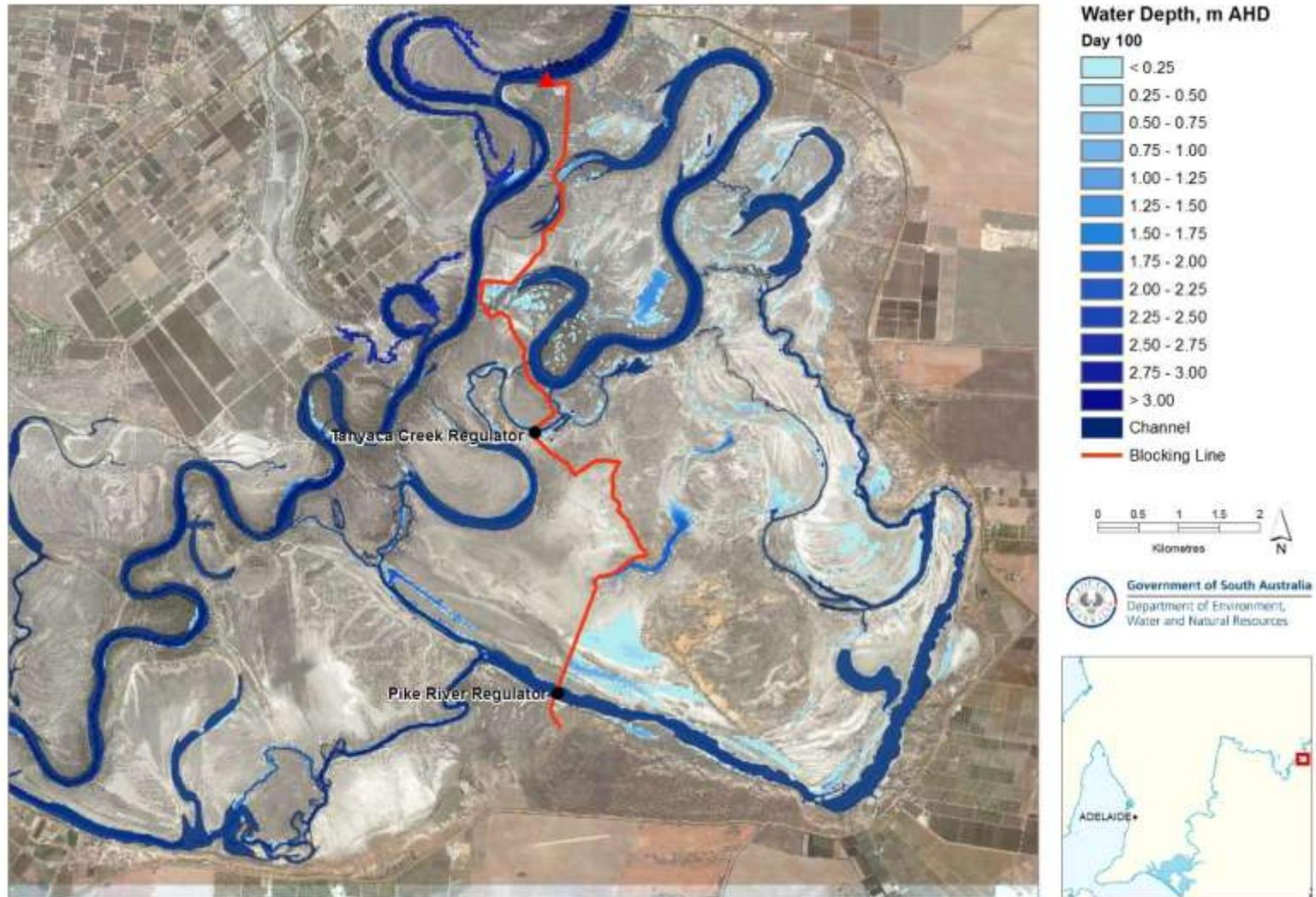
**Figure 9.13 Inundation extent and water depth at Day 100 (water level at Pike Regulator 13.64 m AHD – below typical water level) of managed inundation under Alternative 2 blocking alignment**
