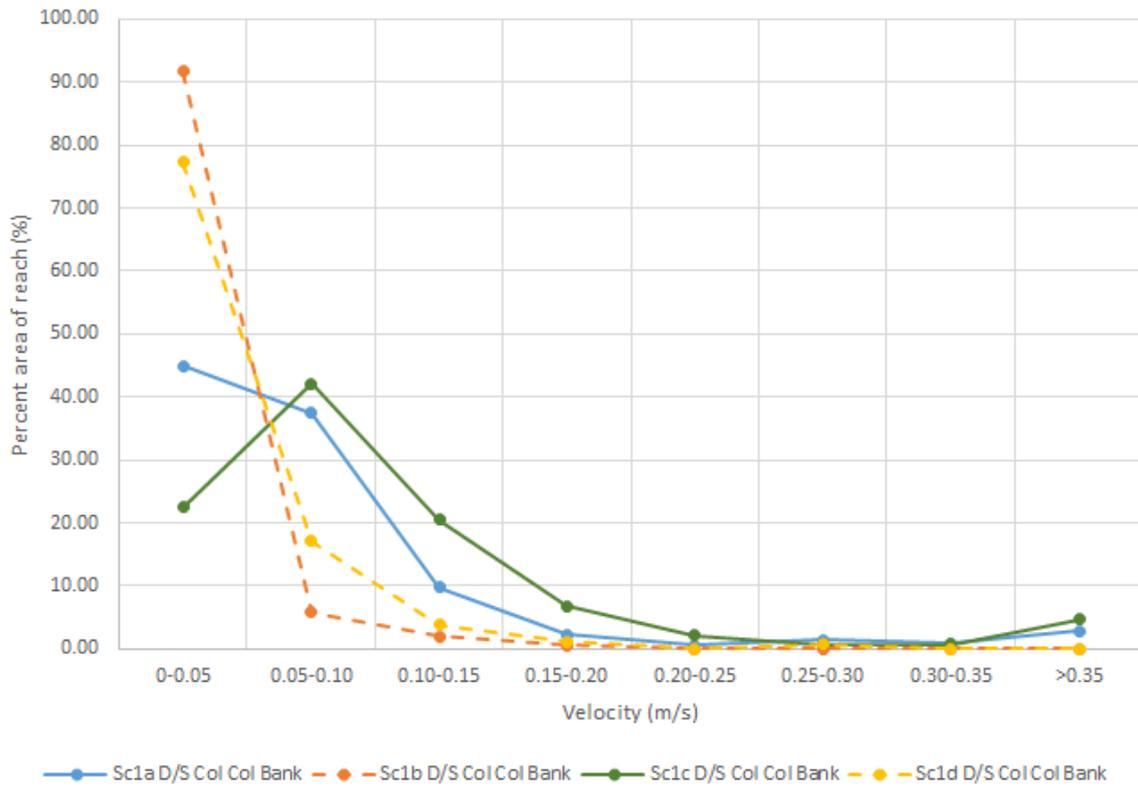
**Figure 3.9 Velocity distribution by percent of reach downstream of existing Col Col Bank (i.e. eastern regulator placement) for Scenarios 1a to 1d (refer to Figure 2.1 for location, enclosed in black dashed line)**
