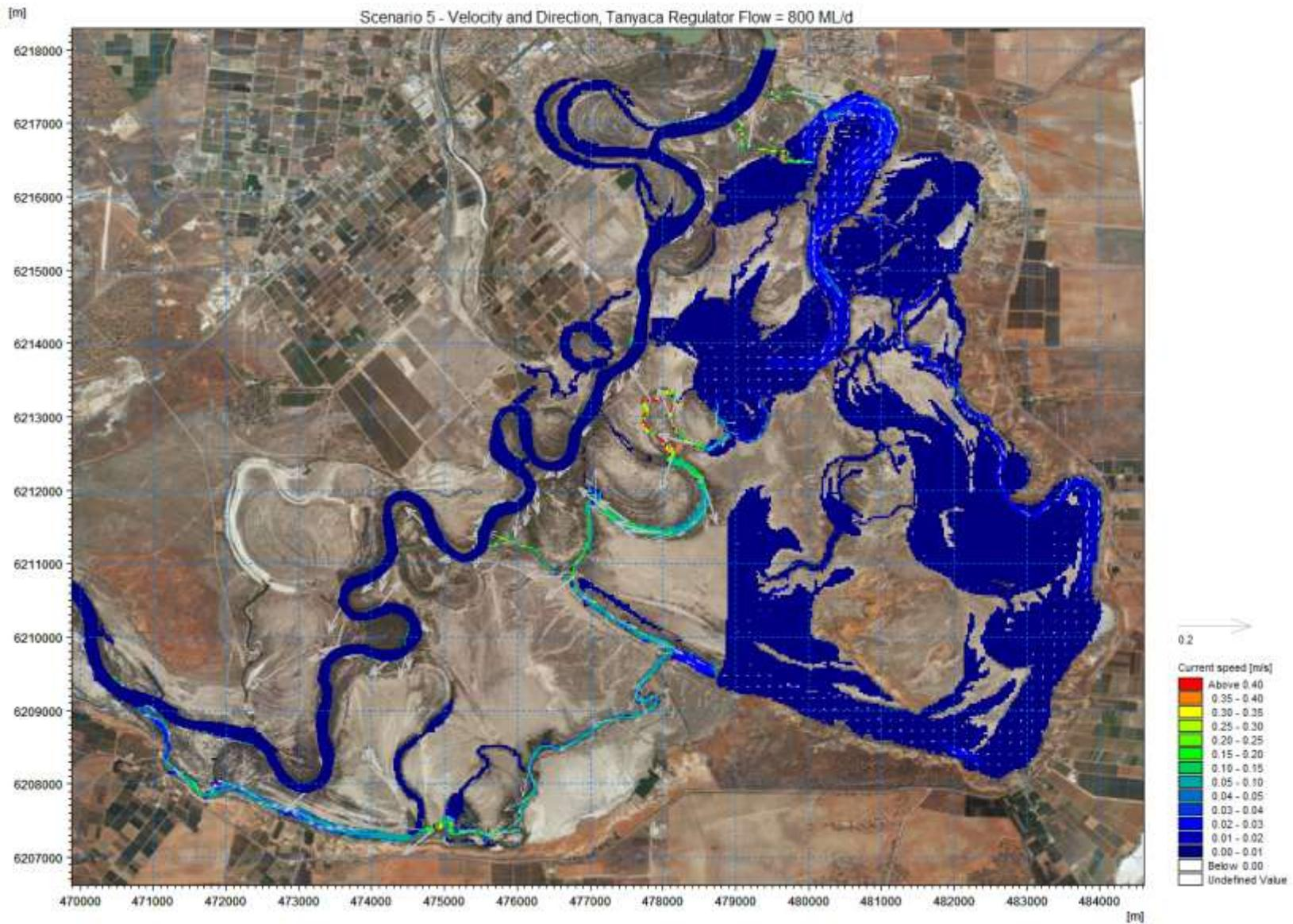
**Figure 7.6 Velocity distribution and flow direction at an inundation level of 16.4 m AHD with alternative Pike River environmental regulator placement and a flow of 800 ML/d through Tanyaca Creek**
