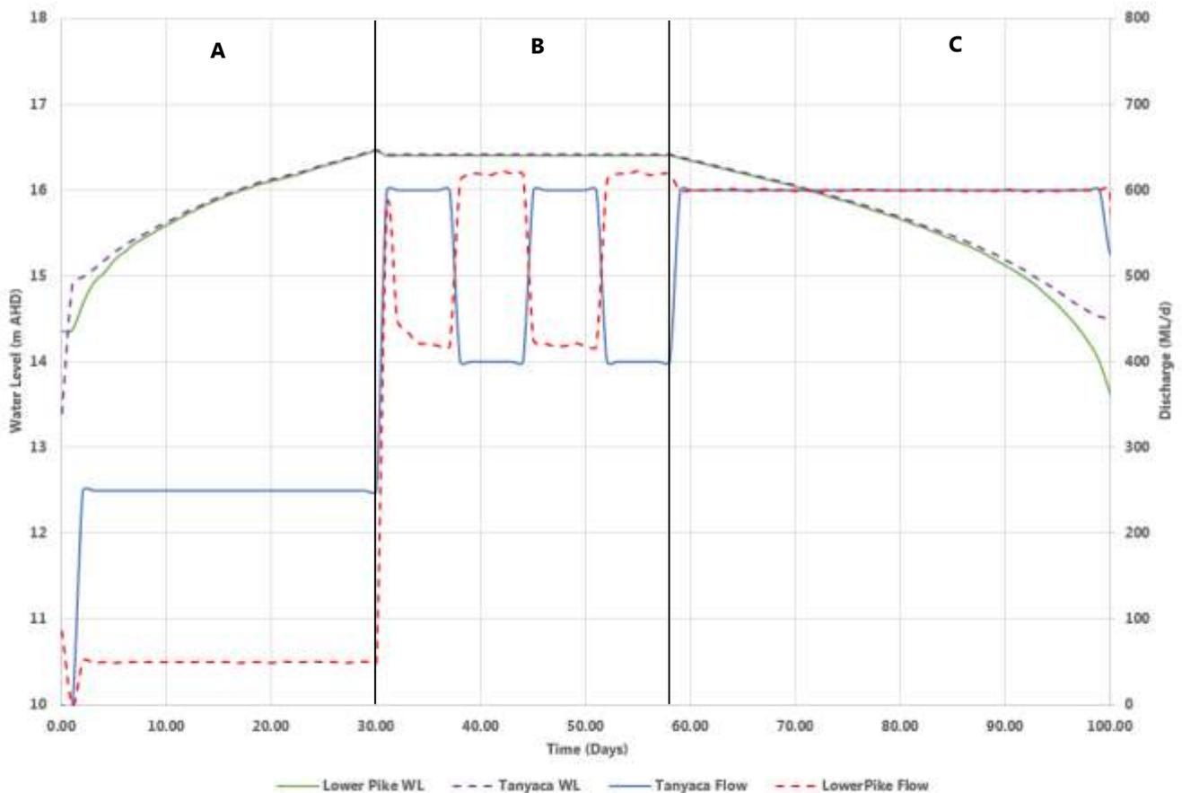
**Figure 9.1 Operating scheme for managed inundation event to 16.4 m AHD full inundation height. Various phases of operation indicated: A – Filling phase; B – Holding phase; and C – Draining phase.**
