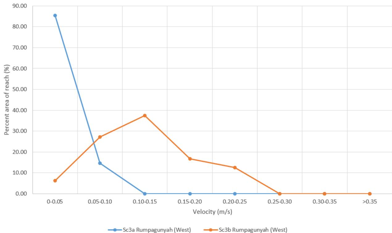
**Figure 5.9 Velocity distribution by percent of reach in western section of Rumpagunyah Creek (between River Murray and Tanyaca outlet into Rumpagunyah) for Scenario 3 simulations (refer to Figure 2.1)**
