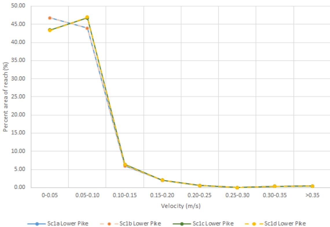
**Figure 3.12 Velocity distribution by percent of reach in Lower Pike (downstream of Rumpagunyah) for Scenarios 1a to 1d (refer to Figure 2.1 for location)**
