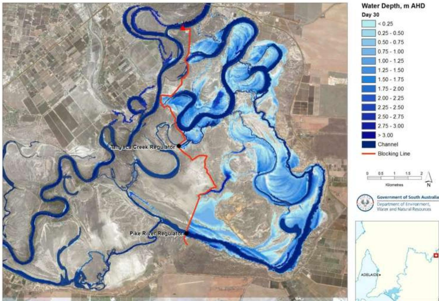
**Figure 9.6 Inundation extent and water depth at Day 30 (water level at Pike Regulator 16.40 m AHD) of managed inundation under Alternative 2 blocking alignment**
