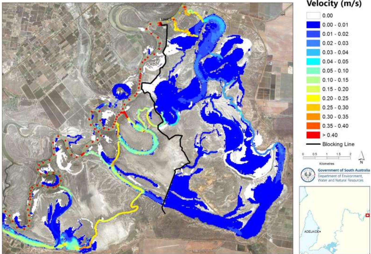
**Figure 10.5 Velocity distribution in Pike Floodplain at flow upstream of Lock 5 at 30 000 ML/d and raised Lock 4 weir pool level at 14.2 m AHD under managed inundation operating conditions**
