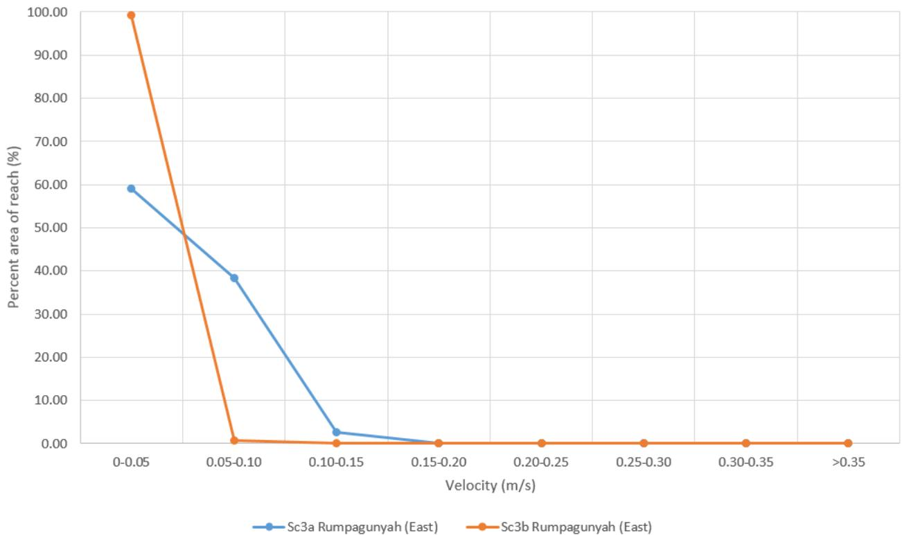
**Figure 5.10 Velocity distribution by percent of reach in eastern section of Rumpagunyah Creek (between Pike River and Tanyaca outlet into Rumpagunyah) for Scenario 3 simulations (refer to Figure 2.1)**
