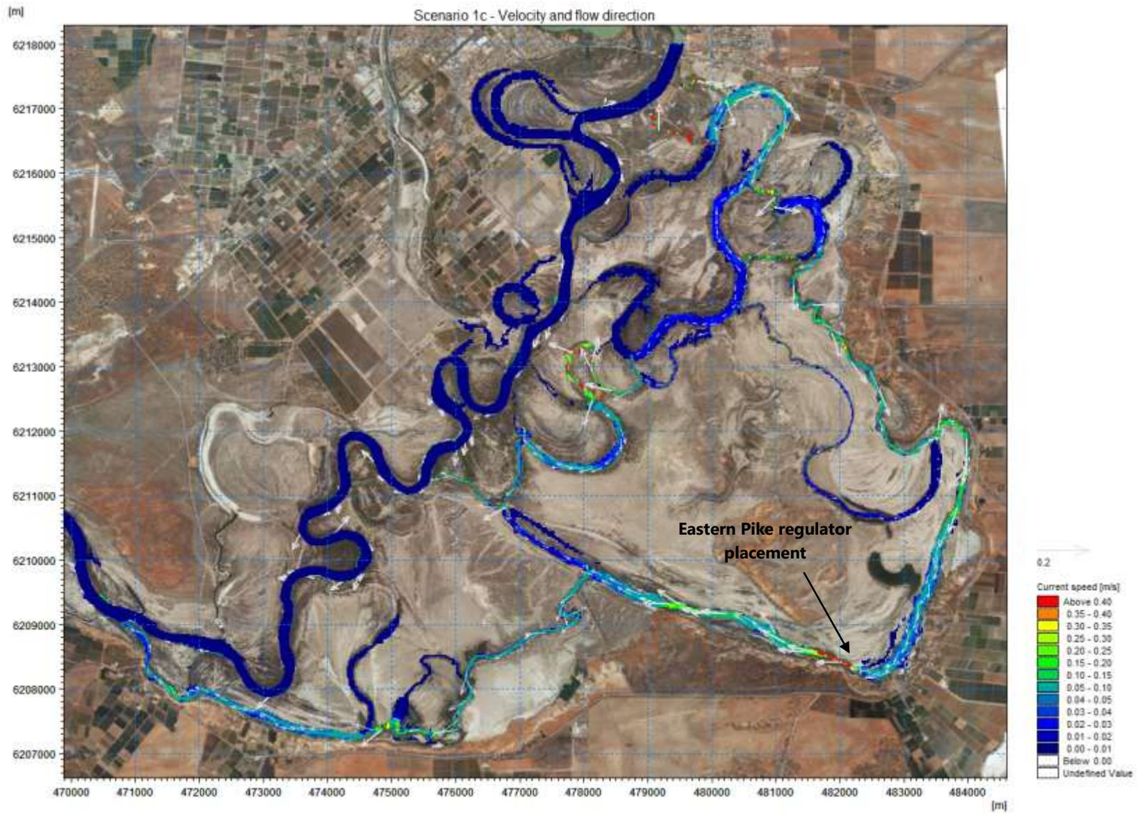
**Figure 3.4 Velocity and flow direction in the Pike Floodplain for Tanyaca regulated flow of 400 ML/d and eastern Pike regulator alternative (Scenario 1c)**
