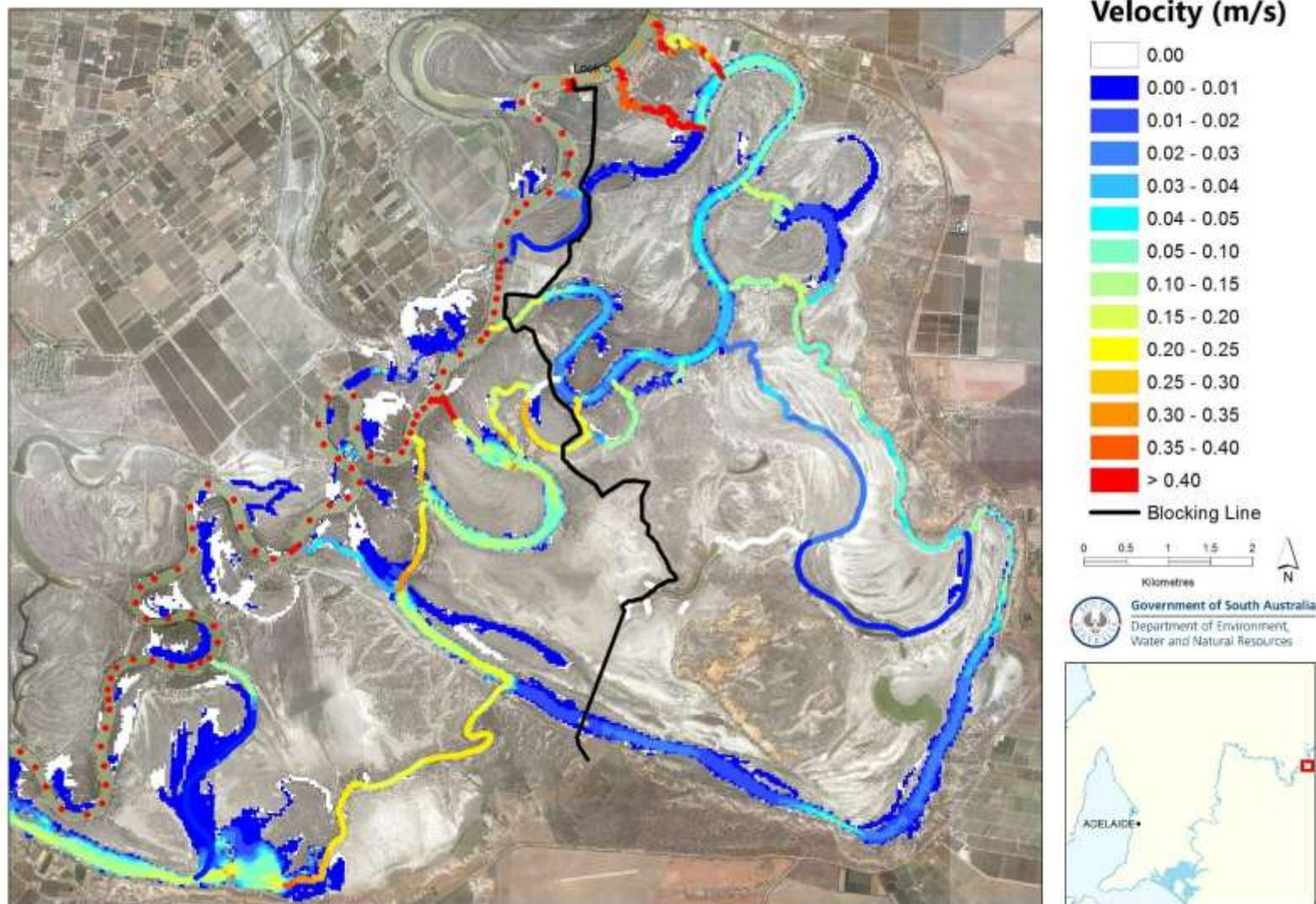
**Figure 10.3 Velocity distribution in Pike Floodplain at flow upstream of Lock 5 at 30 000 ML/d and raised Lock 4 weir pool level at 14.2 m AHD under in-stream flow conditions**
