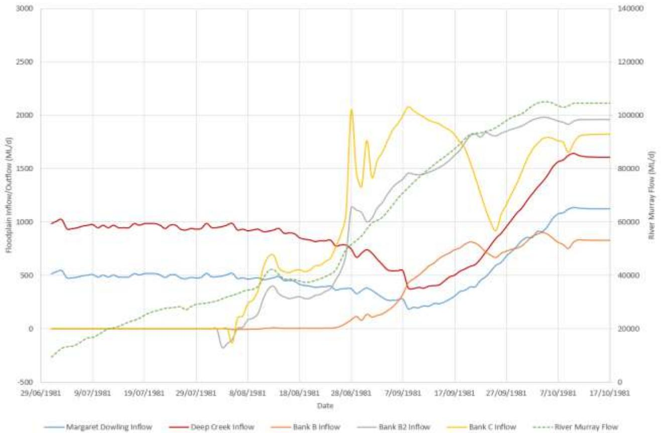
**Figure 8.2** Flows into the floodplain through inlets (total of Margaret Dowling and Deep Creek), Banks B, B2 and C, compared to River Murray flow upstream of Lock 5. Direction of flow at inflow structures indicated by positive (into floodplain) and negative (out of floodplain) values.
