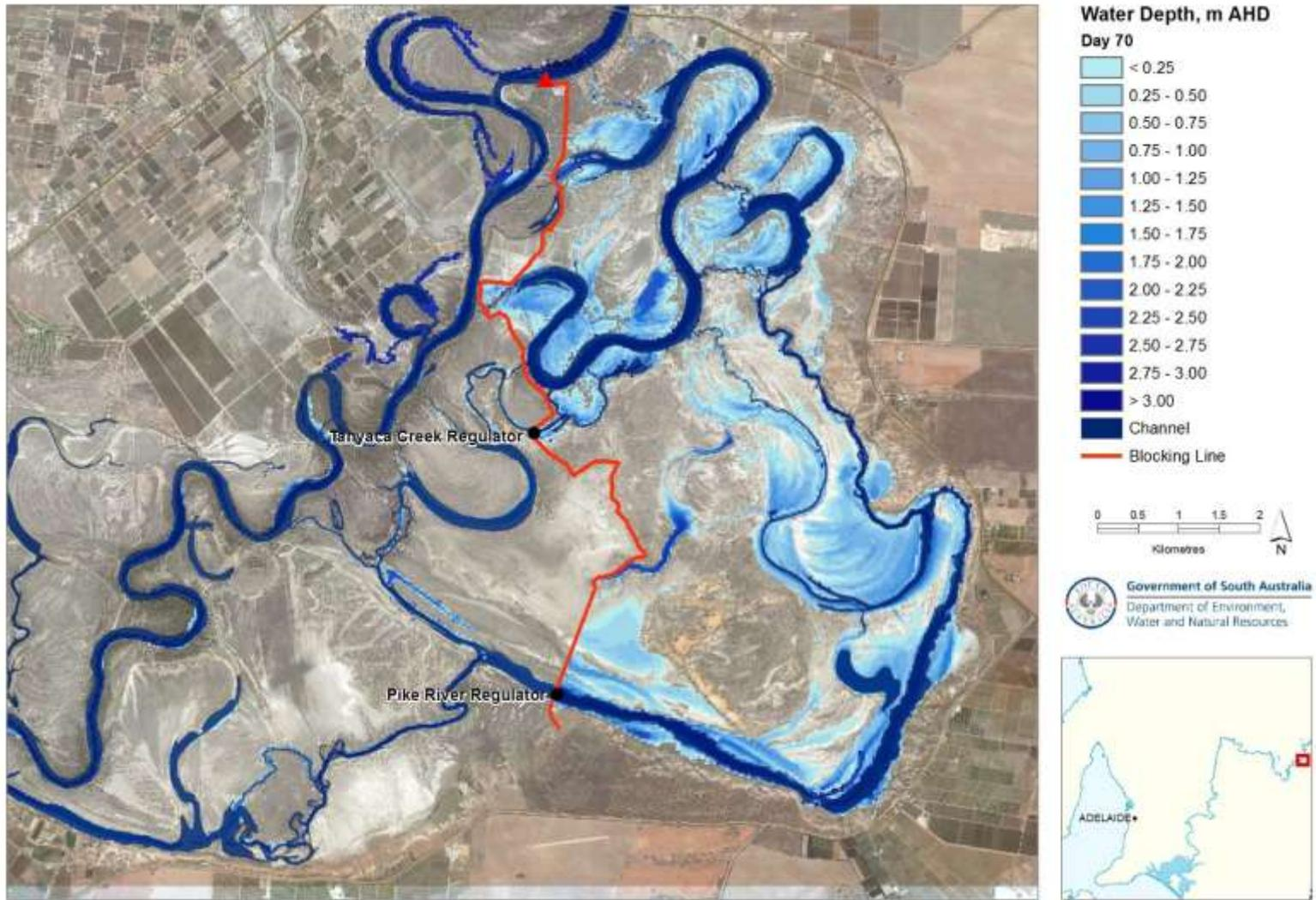
**Figure 9.10 Inundation extent and water depth at Day 70 (water level at Pike Regulator 16.04 m AHD) of managed inundation under Alternative 2 blocking alignment**
