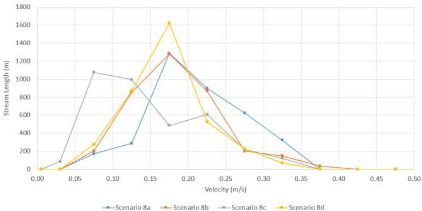
**Figure 10.7 Velocity profiles by stream length for Tanyaca Creek, from Table 10.3**
