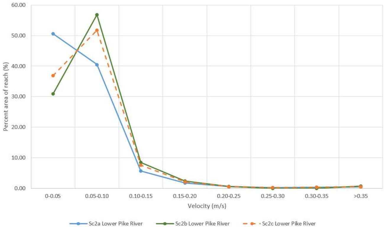
**Figure 4.14 Velocity distribution by percent of reach in Lower Pike River for Scenario 2 simulations (refer to Figure 2.1 for location)**
