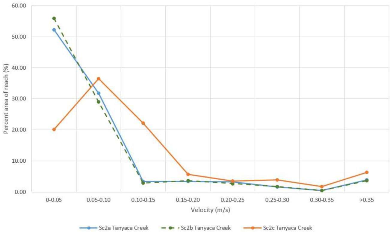
**Figure 4.10 Velocity distribution by percent of reach in Tanyaca Creek for Scenario 2 simulations (refer to Figure 2.1 for location)**
