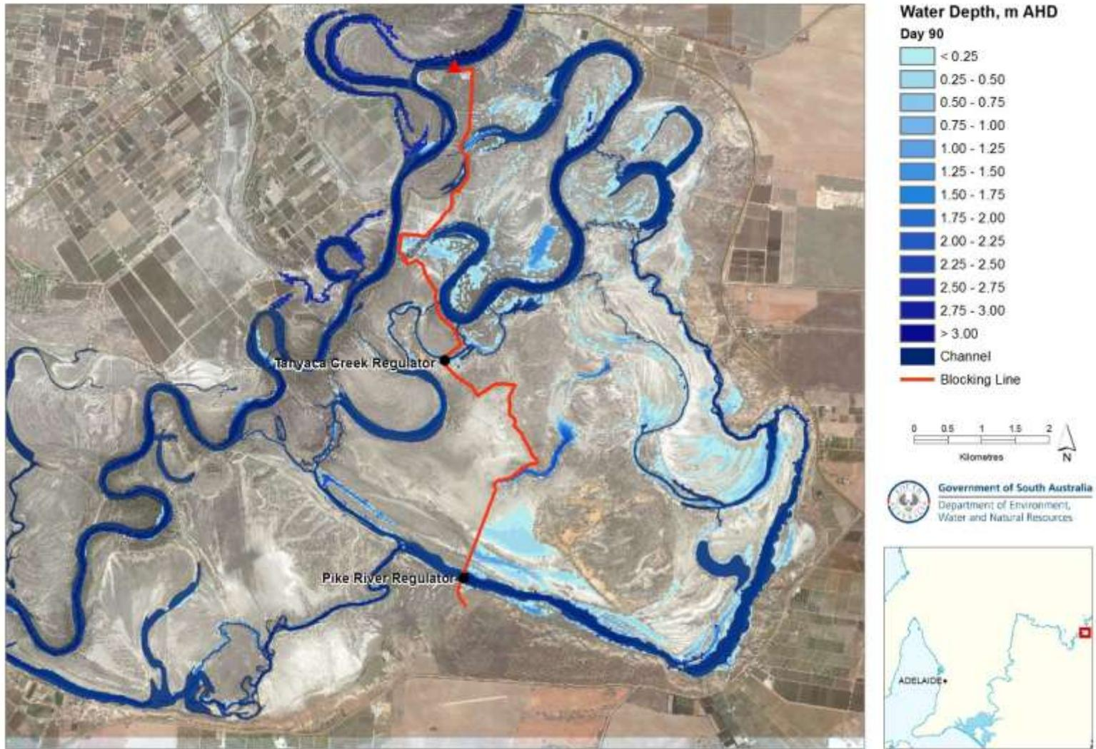
**Figure 9.12 Inundation extent and water depth at Day 90 (water level at Pike Regulator 15.12 m AHD) of managed inundation under Alternative 2 blocking alignment**
