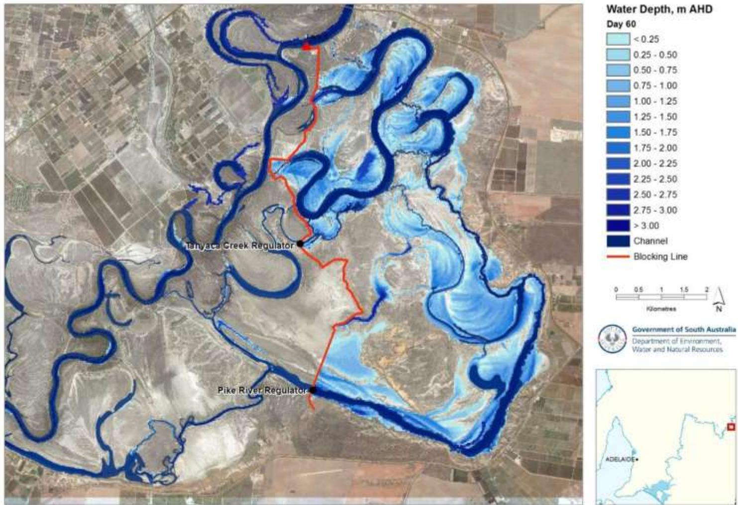
**Figure 9.9 Inundation extent and water depth at Day 60 (water level at Pike Regulator 16.34 m AHD) of managed inundation under Alternative 2 blocking alignment**
