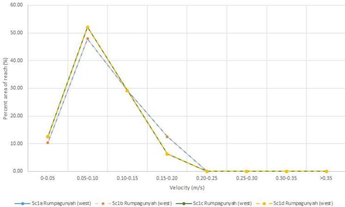
**Figure 3.10 Velocity distribution by percent of reach in western section of Rumpagunyah Creek (between River Murray and Tanyaca outlet into Rumpagunyah) for Scenarios 1a to 1d (refer to Figure 2.1)**
