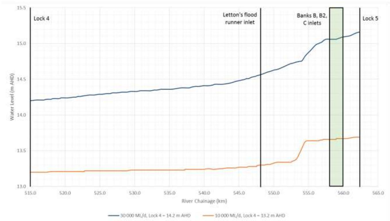
**Figure 10.1 River Murray water level profiles for raised Lock 4 pool level to 14.2 m AHD (flow of 30 000 ML/d above Lock 5) and typical Lock 4 pool level at 13.2 m AHD (flow of 10 000 ML/d above Lock 5)**
