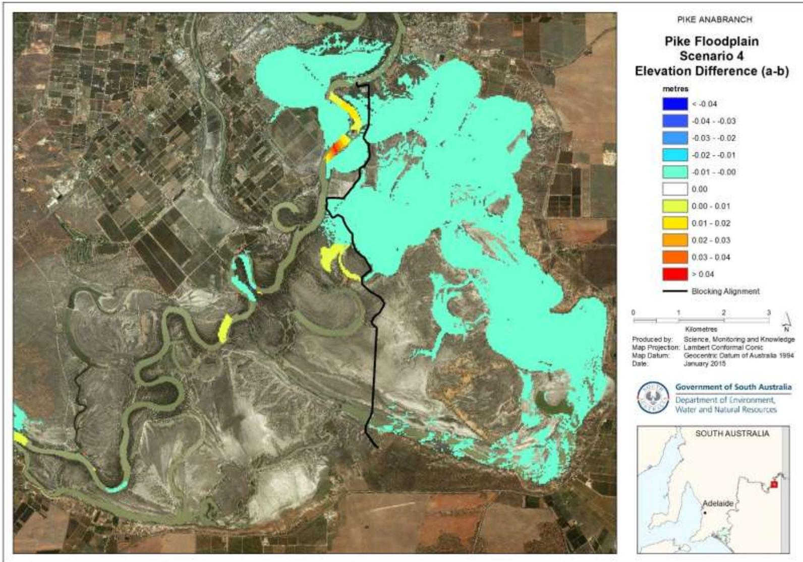
**Figure 6.4 Surface water elevation difference at a River Murray flow of 90 000 ML/d between 100% and 50% concept design regulator sizes**
