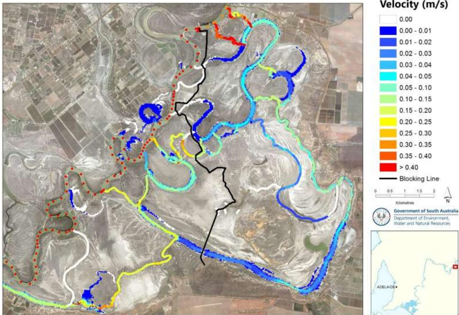
**Figure 10.4 Velocity distribution in Pike Floodplain at flow upstream of Lock 5 at 30 000 ML/d and typical Lock 4 weir pool level at 13.2 m AHD under in-stream flow conditions**
