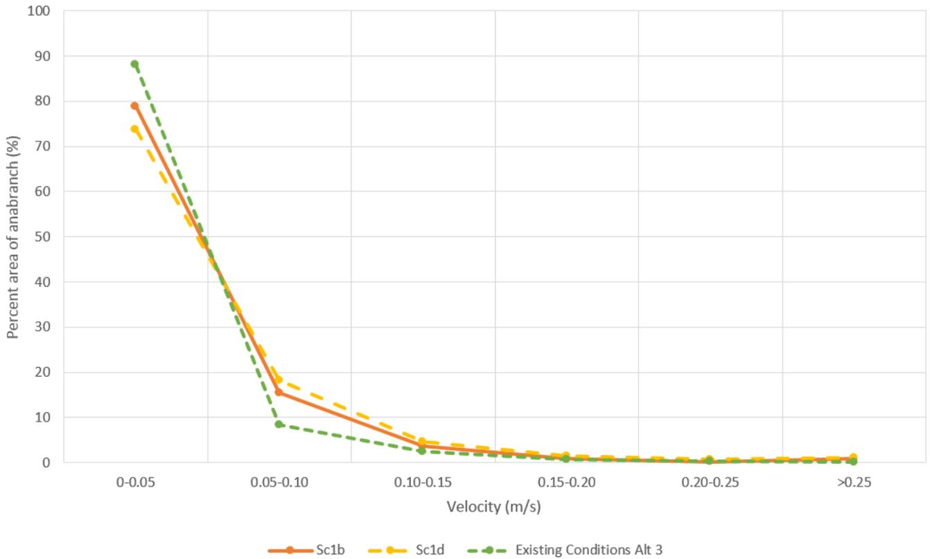
**Figure A.2 Velocity profiles by percent of anabranch for Scenarios 1b and d (i.e. Pike regulator at Alternative 3 downstream location) compared to existing floodplain conditions with an equivalent flow regime**
