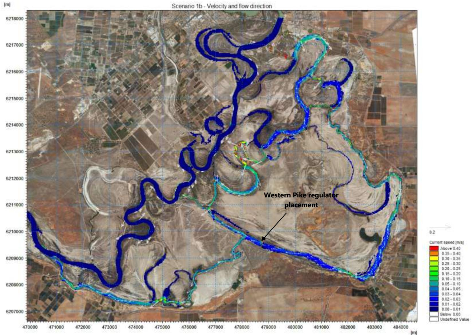
**Figure 3.2 Velocity and flow direction in the Pike Floodplain for Tanyaca regulated flow of 600 ML/d and western Pike regulator alternative (Scenario 1b)**
