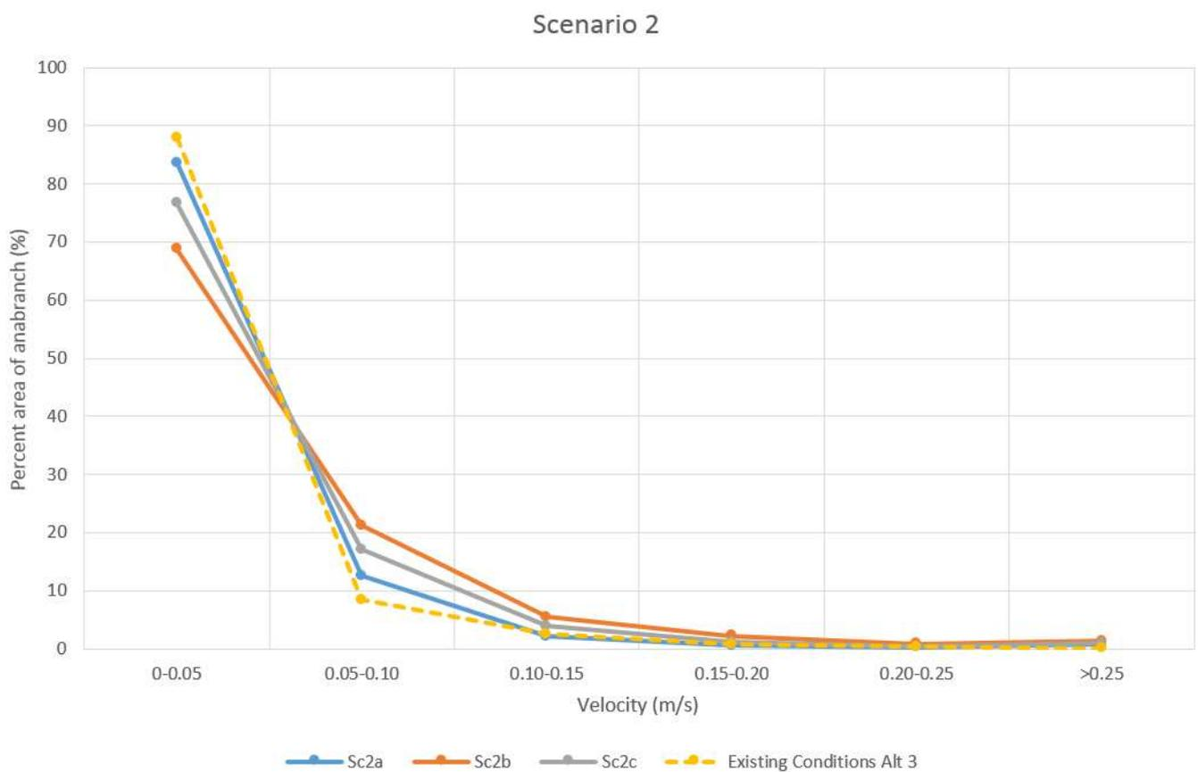
**Figure A.3 Velocity profiles by percent of anabranch for Scenarios 2a to c compared to existing floodplain conditions with an equivalent flow regime**
