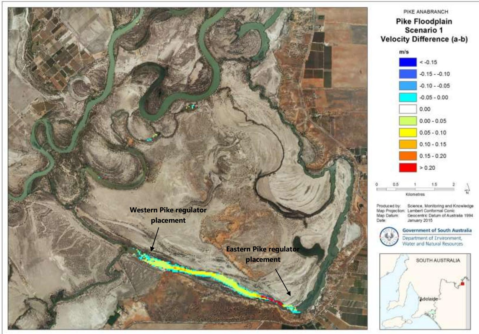
**Figure 3.3 Velocity difference over entire floodplain between alternative Pike regulator placements for a Tanyaca regulated flow of 600 ML/d**
