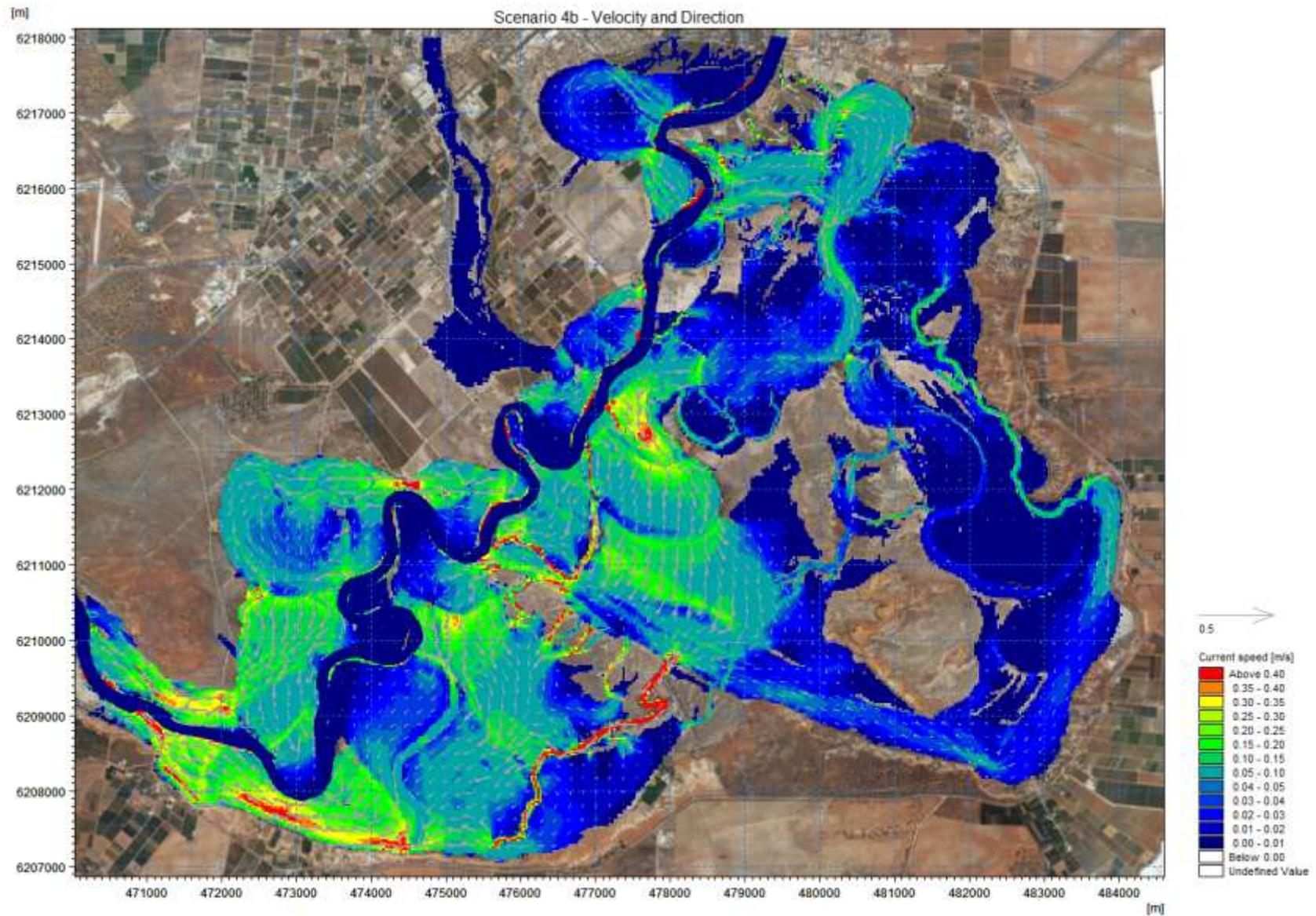
**Figure 6.2 Velocity distribution and direction for River Murray flow of 90 000 ML/d with all structures open. Environmental regulators at Tanyaca and Pike at 50% of concept design size**
