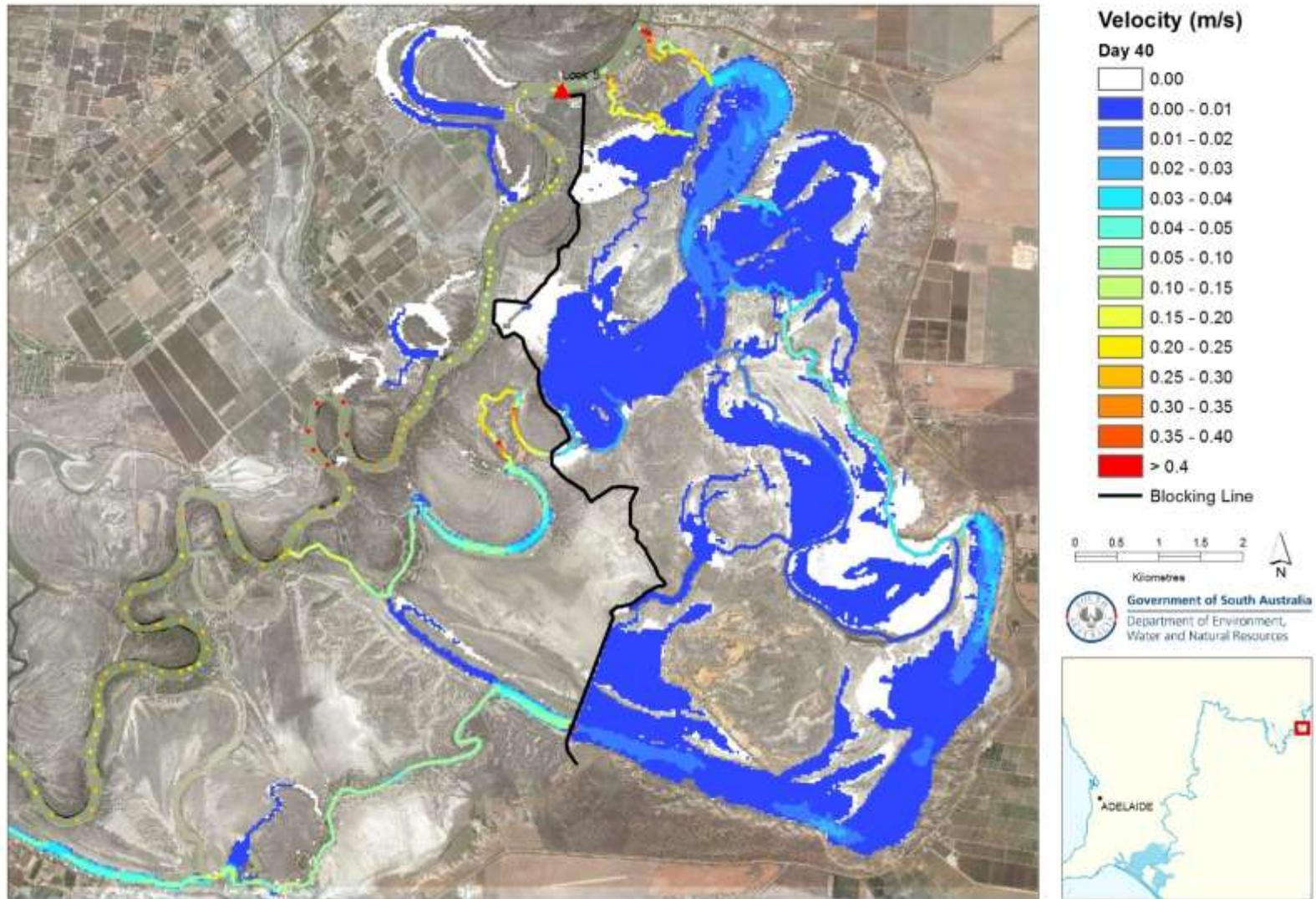
**Figure 9.17 Velocity distribution at Day 40 (water level at Pike Regulator 16.40 m AHD) of managed inundation under Alternative 2 blocking alignment**
