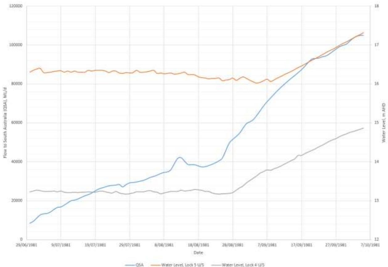
**Figure 8.1 Hydrograph for 1981 flood event, including Flow to South Australia (QSA) and corresponding water levels upstream of Locks 4 and 5**
