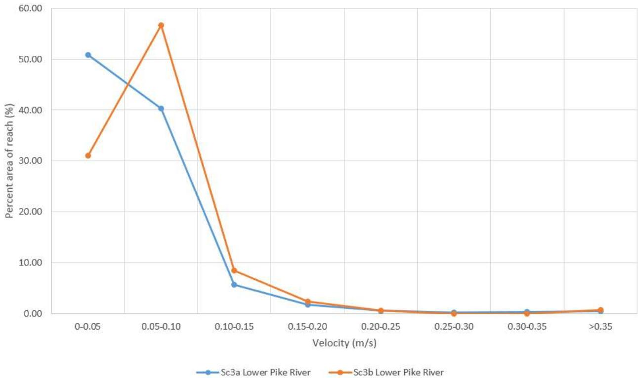
**Figure 5.12 Velocity distribution by percent of reach in Lower Pike River (downstream of Rumpagunyah junction) for Scenario 3 simulations (refer to Figure 2.1 for location)**
