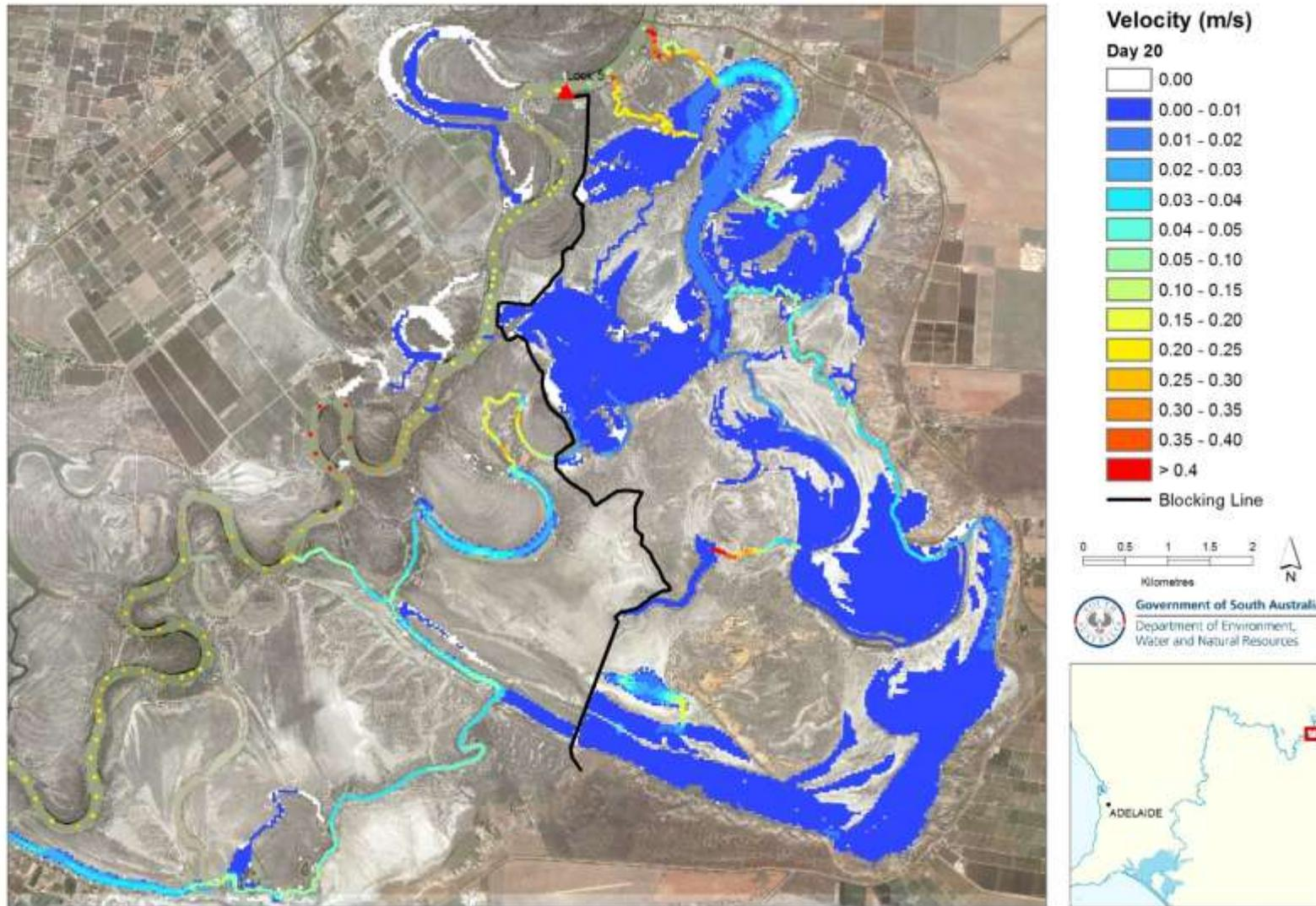
**Figure 9.15 Velocity distribution at Day 20 (water level at Pike Regulator 16.10 m AHD) of managed inundation under Alternative 2 blocking alignment**
