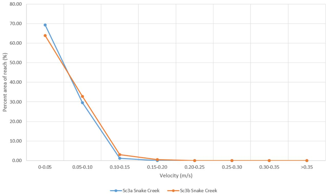
**Figure 5.7 Velocity distribution by percent of reach in Snake Creek for Scenario 3 simulations (refer to Figure 2.1 for location).**
