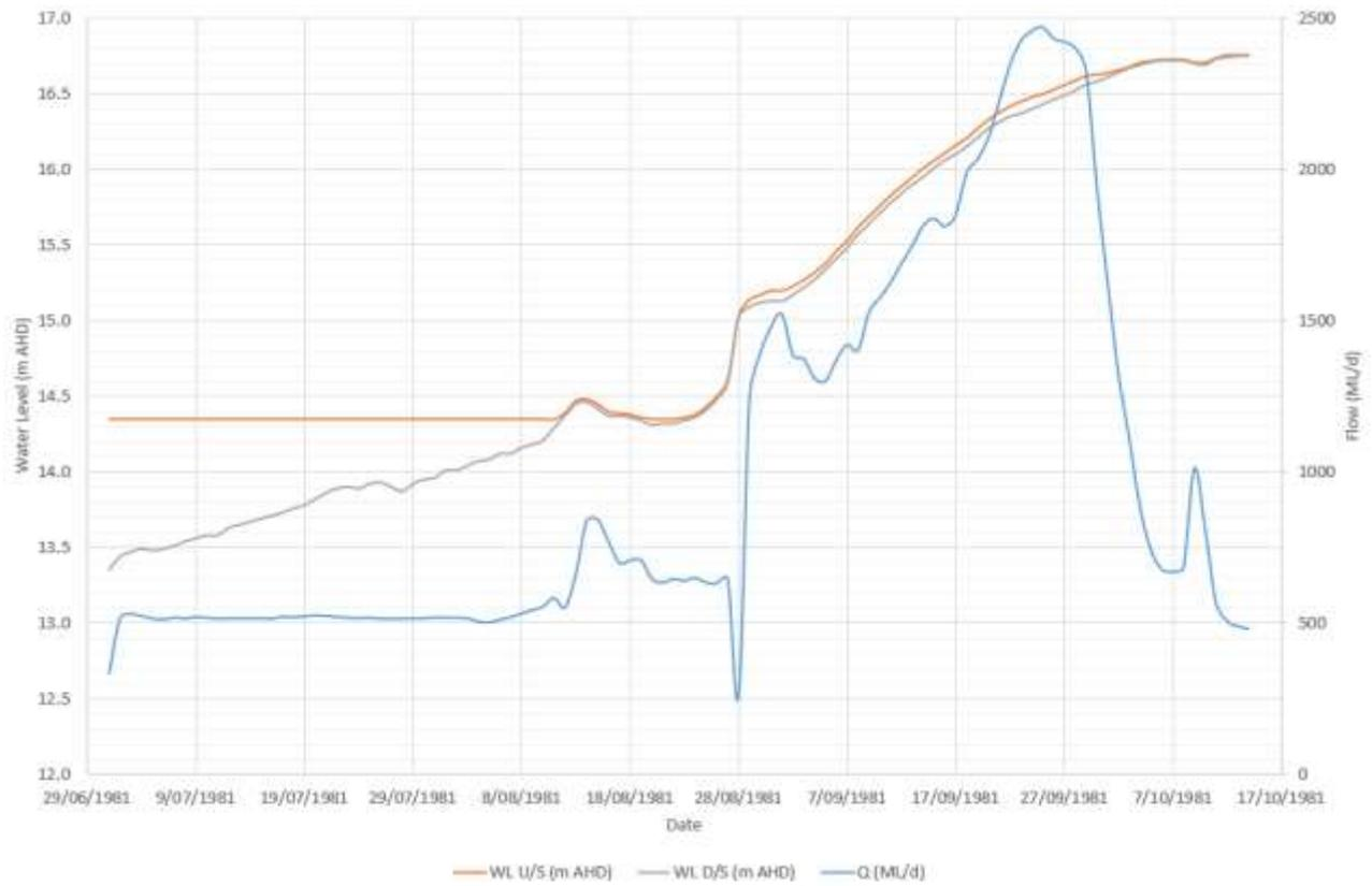
**Figure 8.4 Water levels upstream, downstream and flow through Pike River regulator**
