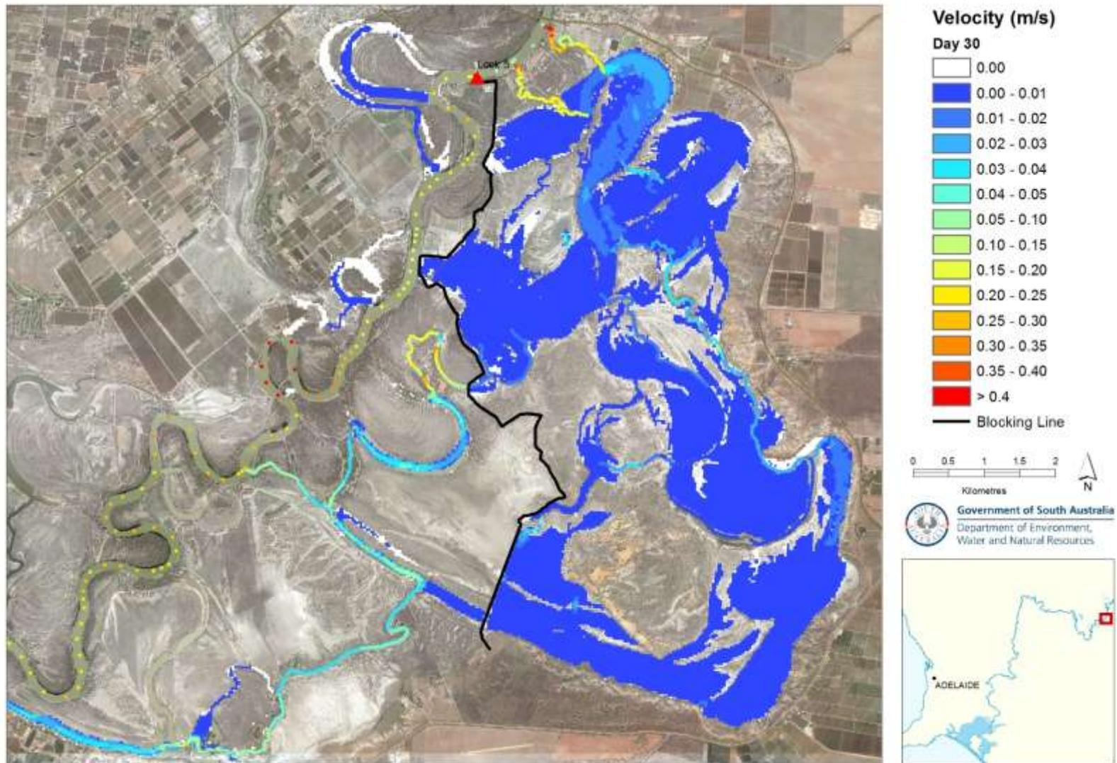
**Figure 9.16 Velocity distribution at Day 30 (water level at Pike Regulator 16.45 m AHD) of managed inundation under Alternative 2 blocking alignment**
