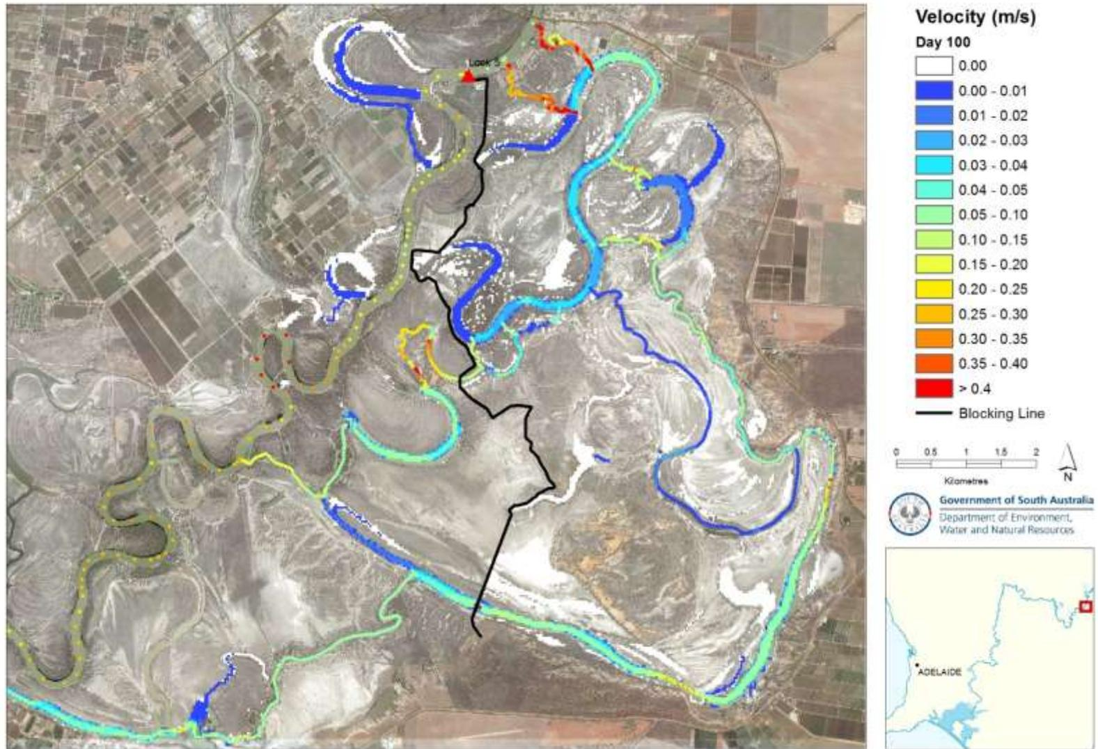
**Figure 9.23 Velocity distribution at Day 100 (water level at Pike Regulator 13.64 m AHD – below typical water level) of managed inundation under Alternative 2 blocking alignment**
