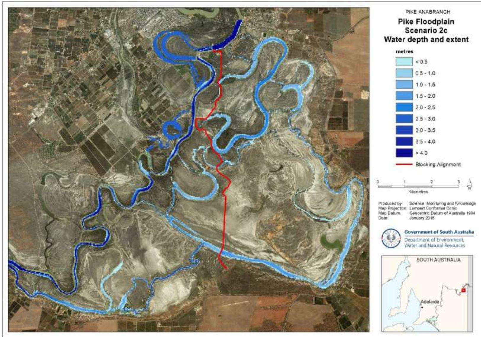
**Figure 4.5 Water depth and extent for an inflow of 1200 ML/d and Tanyaca flow of 800 ML/d (Scenario 2c)**
