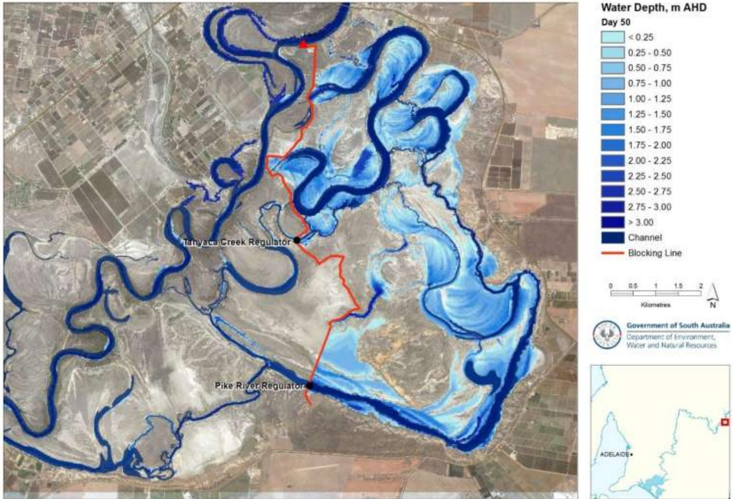
**Figure 9.8 Inundation extent and water depth at Day 50 (water level at Pike Regulator 16.40 m AHD) of managed inundation under Alternative 2 blocking alignment**
