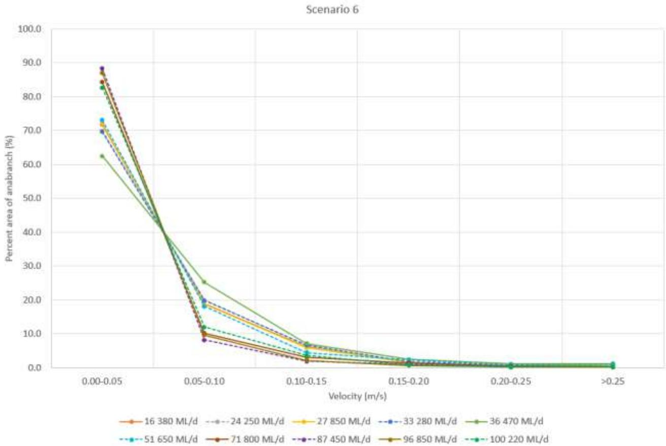
**Figure A.7 Velocity profiles by percent of anabranch for Scenario 6 for various River Murray flows, corresponding to 10-day increments of the hydrograph**
