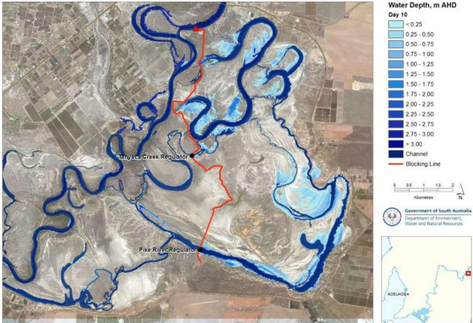
**Figure 9.4 Inundation extent and water depth at Day 10 (water level at Pike Regulator 15.59 m AHD) of managed inundation under Alternative 2 blocking alignment**
