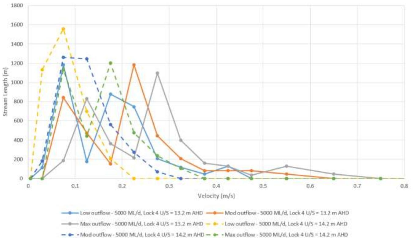
Figure 11.4 Tanyaca Creek velocity profiles by stream length, river flow 5000 ML/d, from Table 11.4
