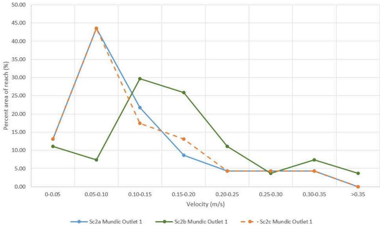
**Figure 4.7 Velocity distribution by percent of reach in Mundic Creek Northern Outlet for Scenario 2 simulations (refer to Figure 2.1 for location)**
