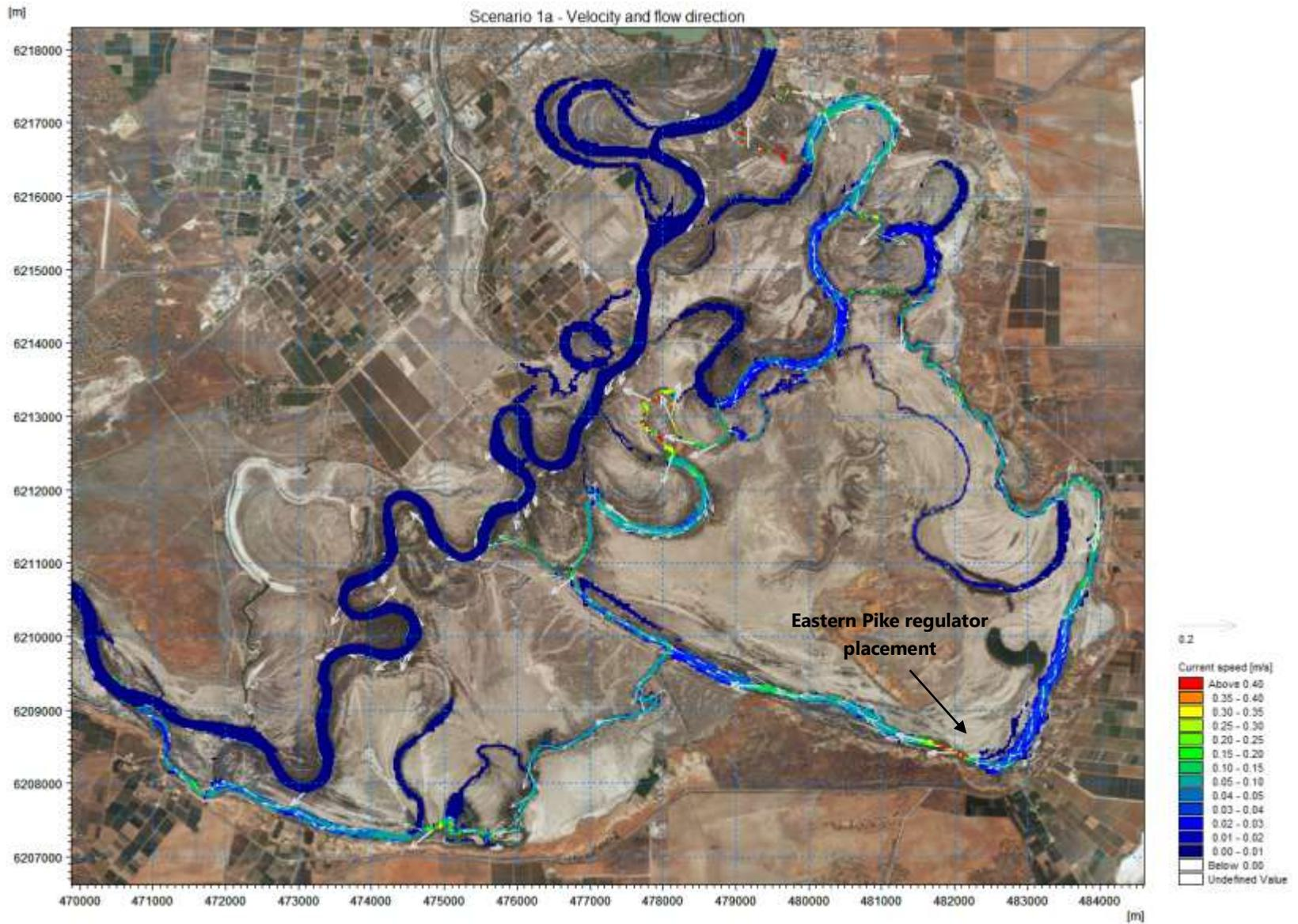
**Figure 3.1 Velocity and flow direction in the Pike Floodplain for Tanyaca regulated flow of 600 ML/d and eastern Pike regulator alternative (Scenario 1a)**
