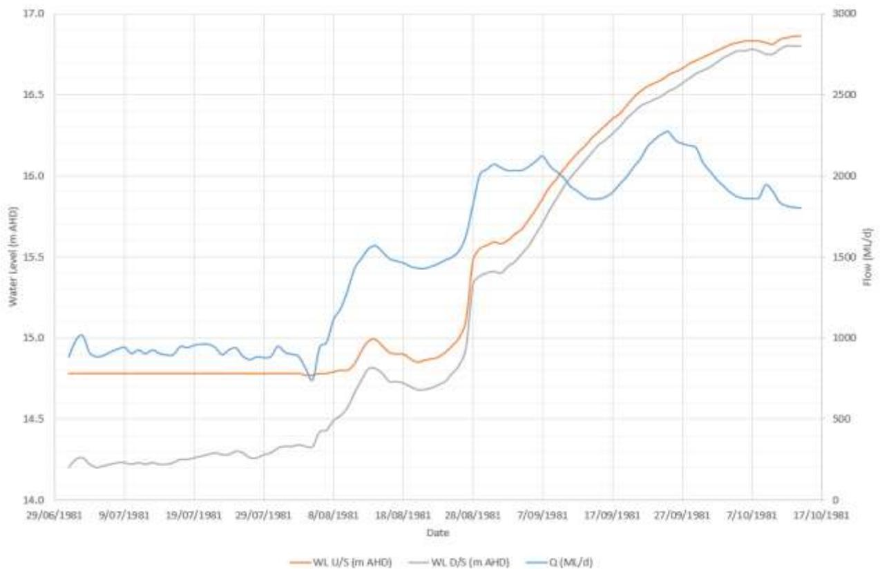
**Figure 8.3** Water levels upstream, downstream and flow through Tanyaca Creek regulator
