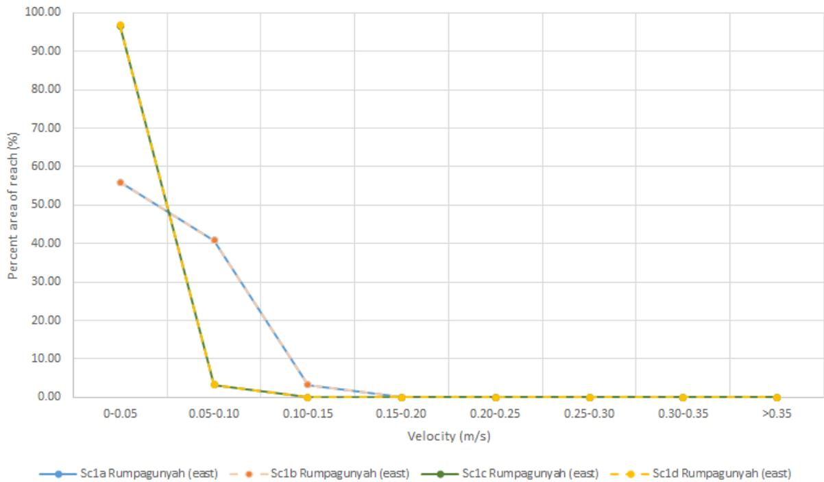
**Figure 3.11 Velocity distribution by percent of reach in eastern section of Rumpagunyah Creek (between Pike River and Tanyaca outlet into Rumpagunyah) for Scenarios 1a to 1d (refer to Figure 2.1 for location)**
