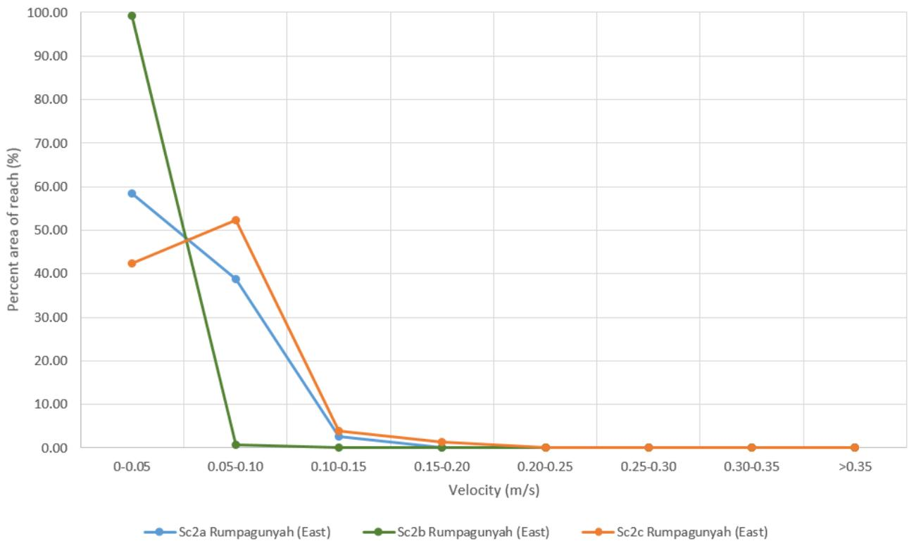
**Figure 4.12 Velocity distribution by percent of reach in eastern section of Rumpagunyah Creek (between Pike River and Tanyaca outlet into Rumpagunyah) for Scenario 2 simulations (refer to Figure 2.1)**
