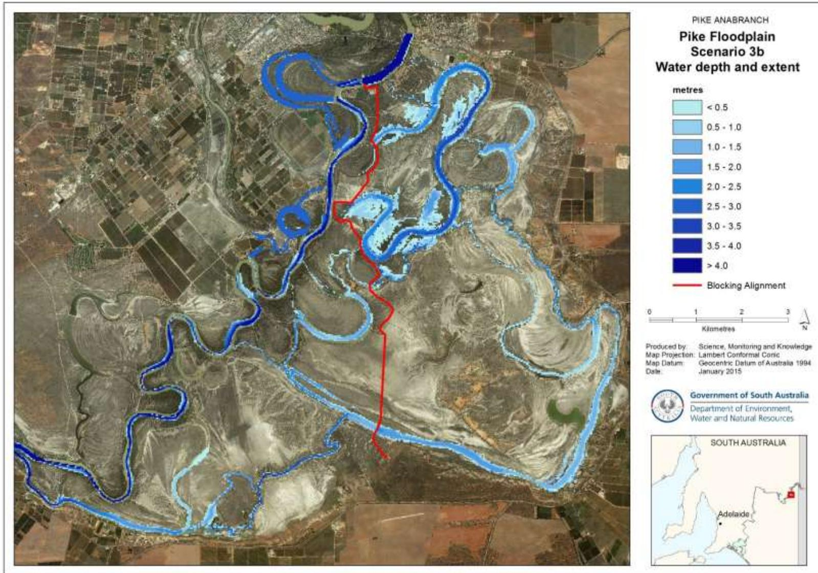
**Figure 5.3 Water depth and extent for an inflow of 1200 ML/d and minor regulators on Mundic Creek outlets passing 800 ML/d (Scenario 3b)**
