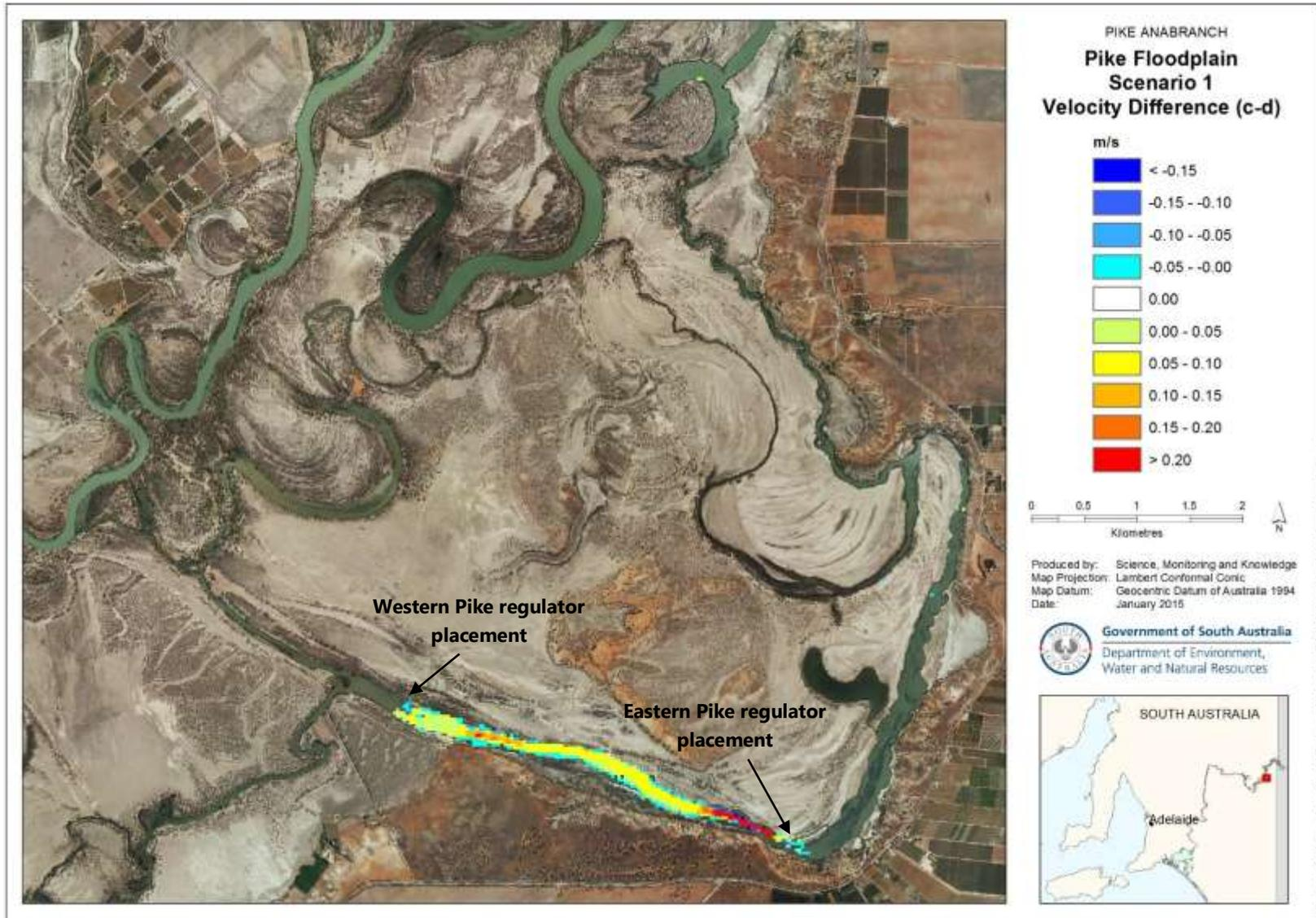
**Figure 3.6 Velocity difference over entire floodplain between alternative Pike regulator placements for a Tanyaca regulated flow of 400 ML/d**
