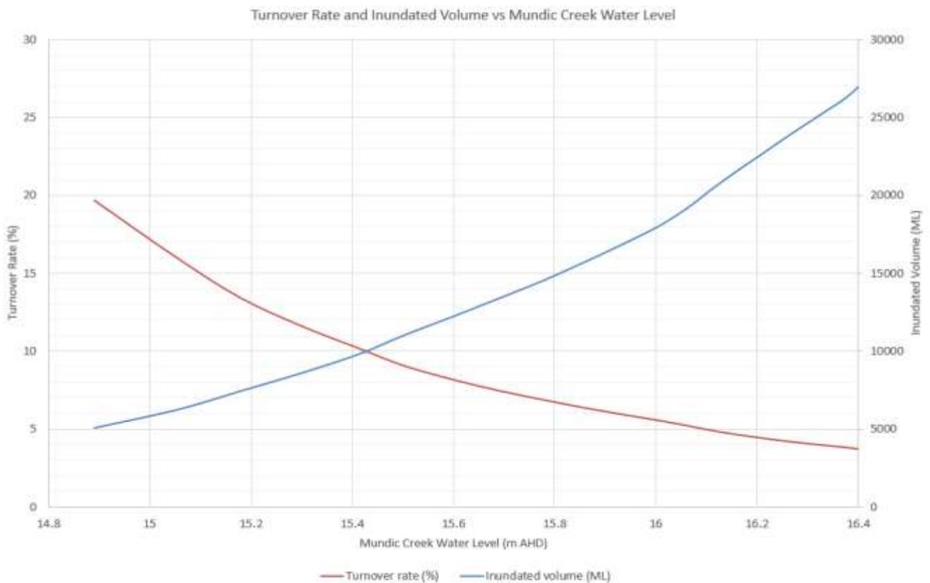
**Figure 7.8 Overall turnover rate and impounded volume versus inundation height at Mundic Creek**
