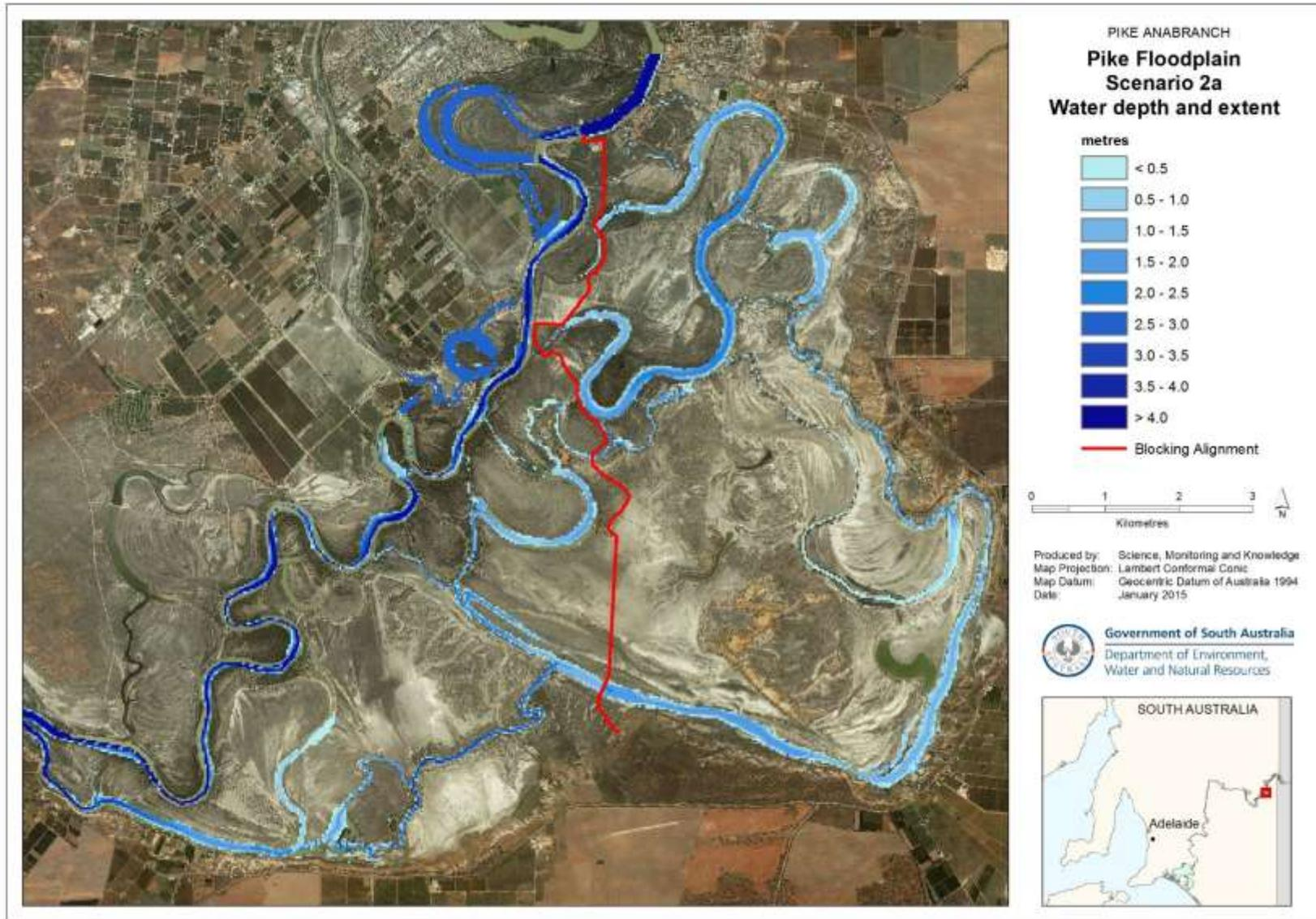
**Figure 4.1 Water depth and extent for an inflow of 800 ML/d and Tanyaca flow of 400 ML/d (Scenario 2a)**
