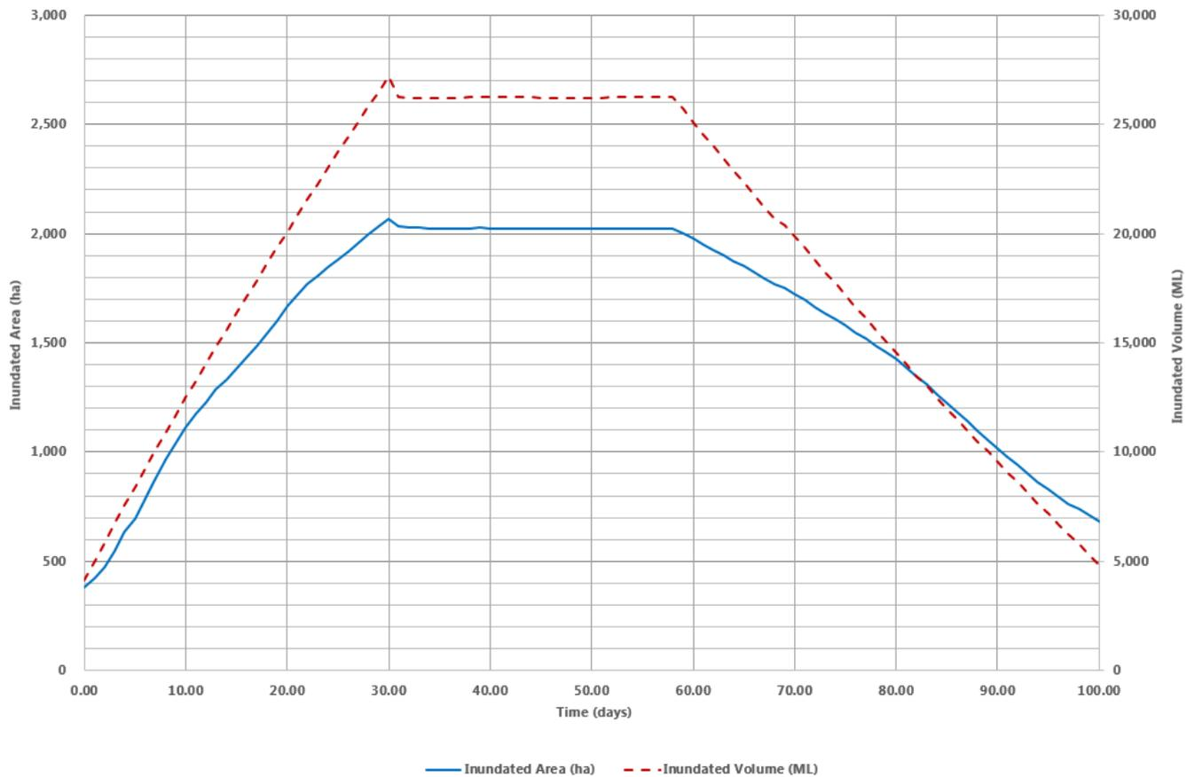
**Figure 9.2 Inundated area and volume during period of operation.**
