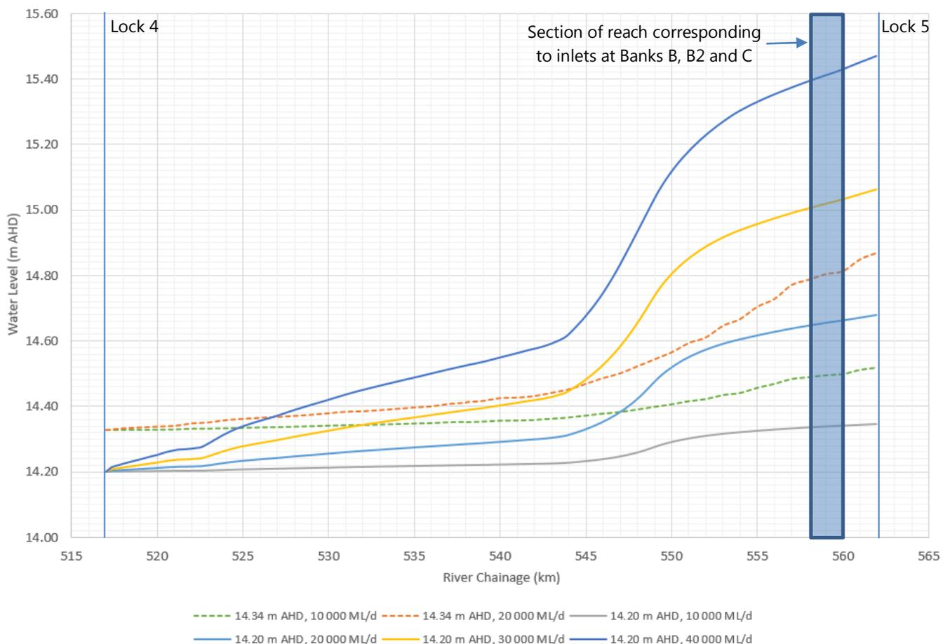
**Figure 7.2 Modelled water levels between Locks 4 and 5 for raised Lock 4 weir pool levels of 14.34 m AHD (Macky and Bloss, 2012) and 14.20 m AHD (McCullough et al., 2016), at various River Murray flows downstream of Lock 5. Locations of Locks 4 and 5, and section of reach corresponding to inlets at Banks B, B2 and C are indicated.**
