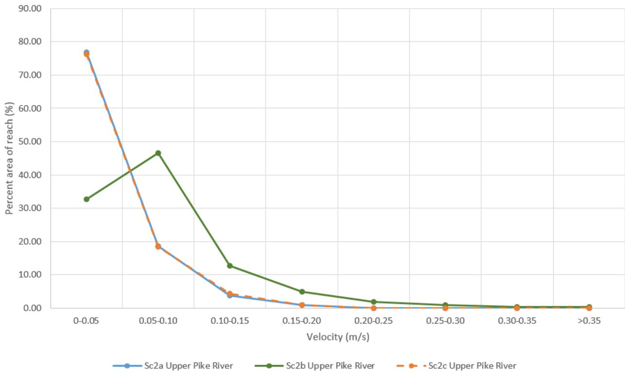
**Figure 4.13 Velocity distribution by percent of reach in Upper Pike River for Scenario 2 simulations (refer to Figure 2.1 for location)**
