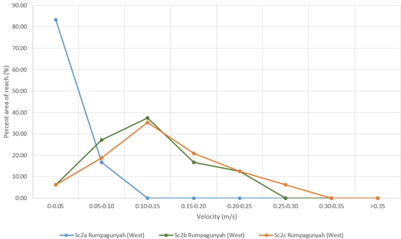
**Figure 4.11 Velocity distribution by percent of reach in western section of Rumpagunyah Creek (between River Murray and Tanyaca outlet into Rumpagunyah) for Scenario 2 simulations (refer to Figure 2.1)**
