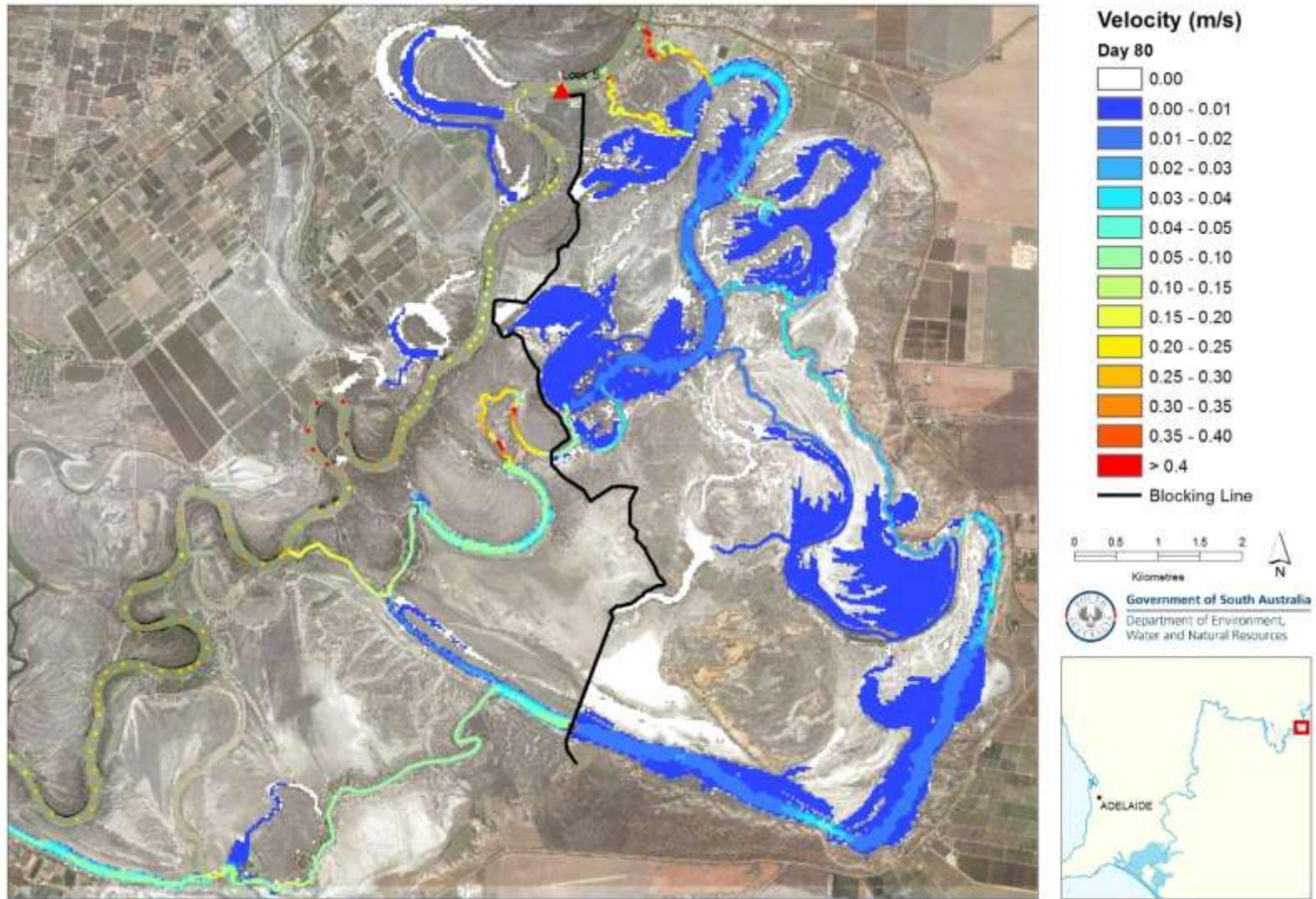
**Figure 9.21 Velocity distribution at Day 80 (water level at Pike Regulator 15.66 m AHD) of managed inundation under Alternative 2 blocking alignment**
