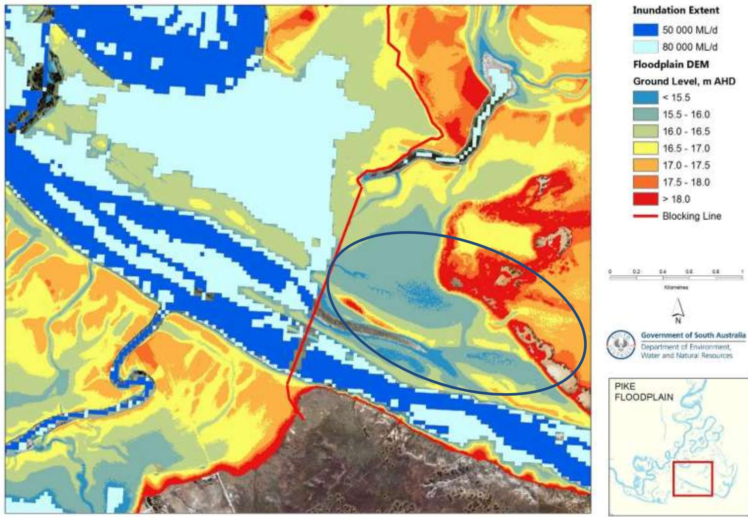
**Figure 8.5** Inundation extents at River Murray flows of 50 000 ML/d (water level at Pike regulator of 14.61 m AHD) and 80 000 ML/d (water level at Pike River regulator of 15.95 m AHD), with reference to ground level elevation from Digital Elevation Model (DEM) of floodplain. Approximate area prevented from inundation by blocking bank is encircled in dark blue.
