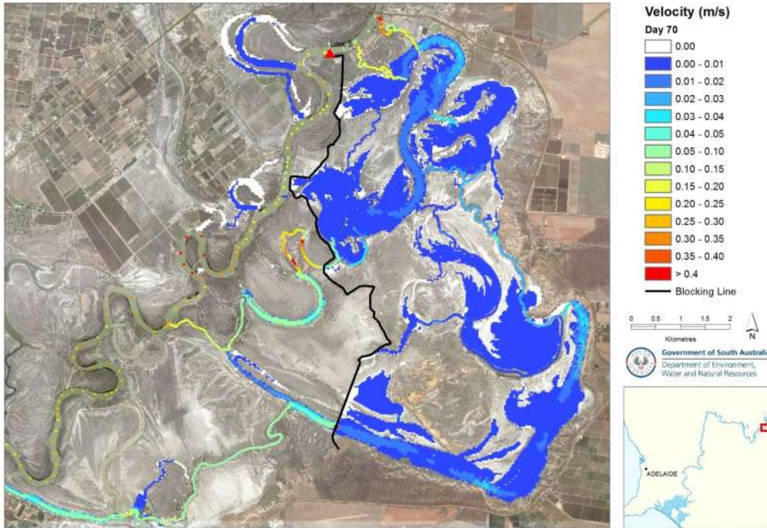
**Figure 9.20 Velocity distribution at Day 70 (water level at Pike Regulator 16.04 m AHD) of managed inundation under Alternative 2 blocking alignment**
