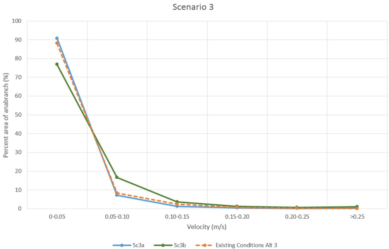
**Figure A.4 Velocity profiles by percent of anabranch for Scenarios 3a and b compared to existing floodplain conditions with an equivalent flow regime**
