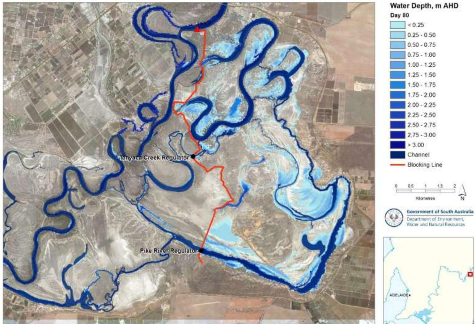
**Figure 9.11 Inundation extent and water depth at Day 80 (water level at Pike Regulator 15.66 m AHD) of managed inundation under Alternative 2 blocking alignment**
