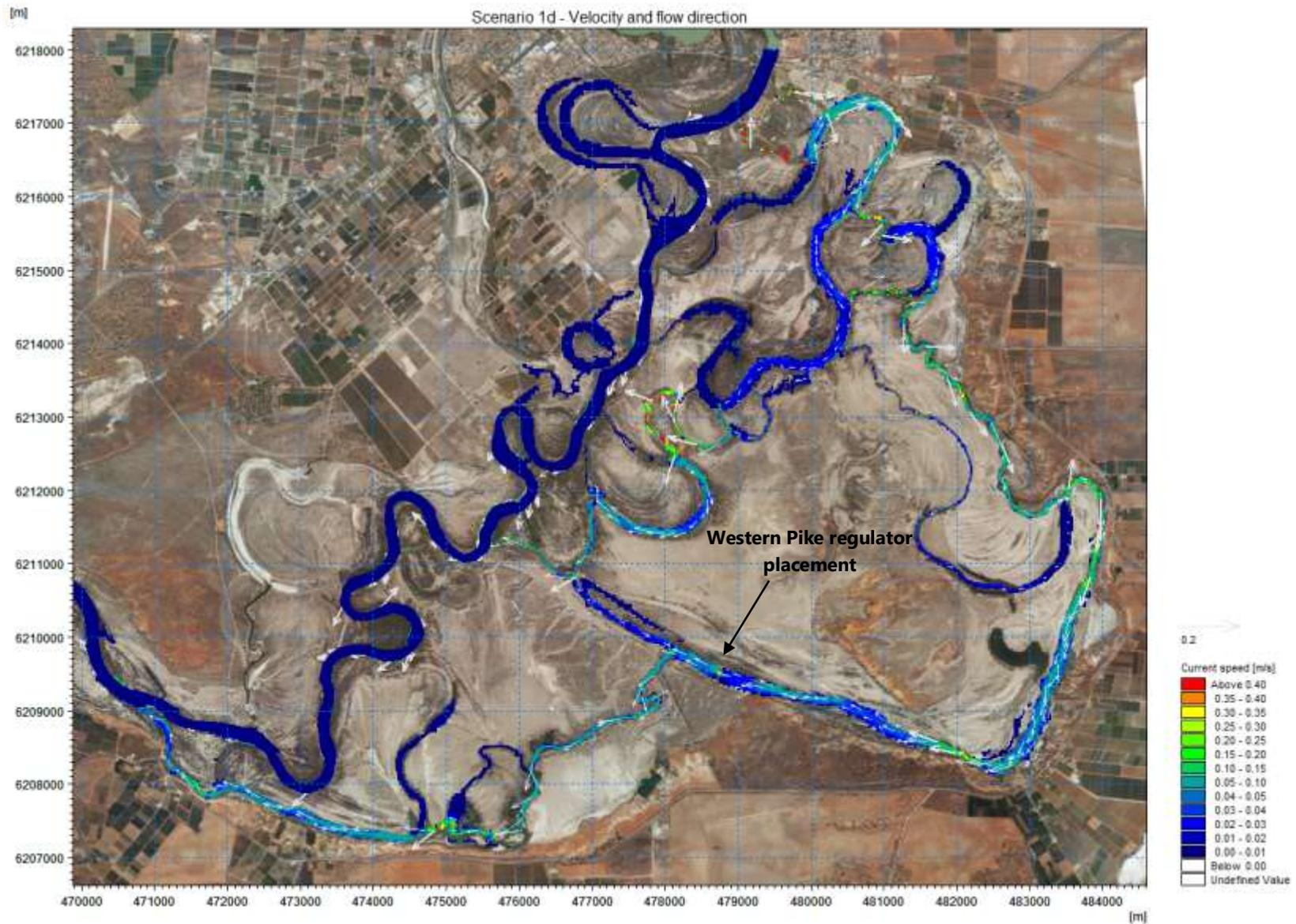
**Figure 3.5 Velocity and flow direction in the Pike Floodplain for Tanyaca regulated flow of 400 ML/d and western Pike regulator alternative (Scenario 1d)**
