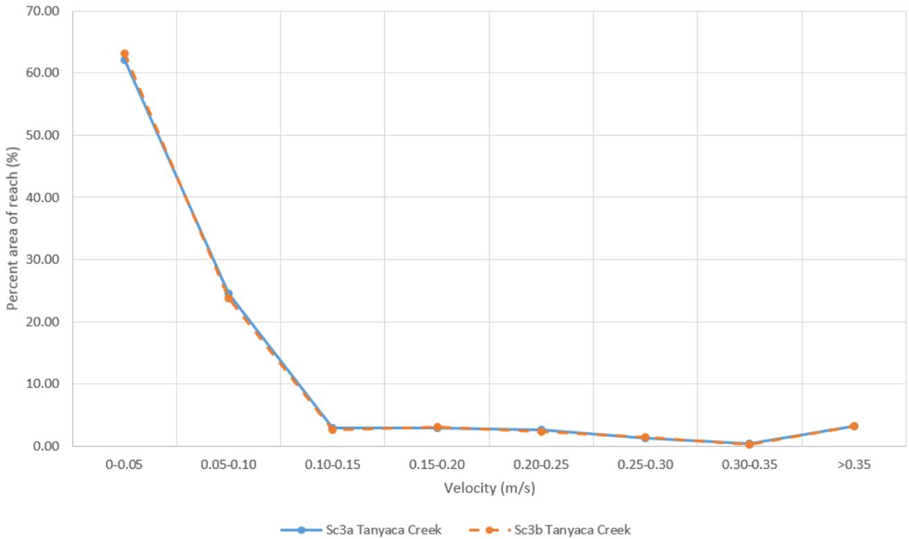
**Figure 5.8 Velocity distribution by percent of reach in Tanyaca Creek for Scenario 3 simulations (refer to Figure 2.1 for location)**
