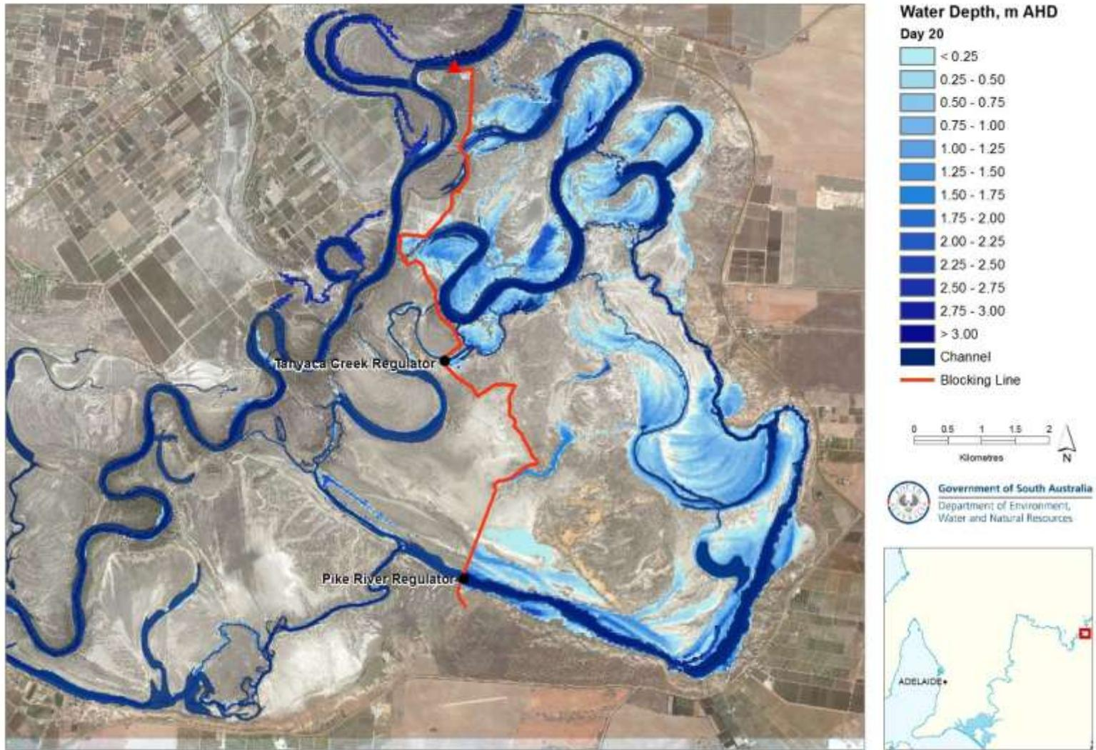
**Figure 9.5 Inundation extent and water depth at Day 20 (water level at Pike Regulator 16.10 m AHD) of managed inundation under Alternative 2 blocking alignment**
