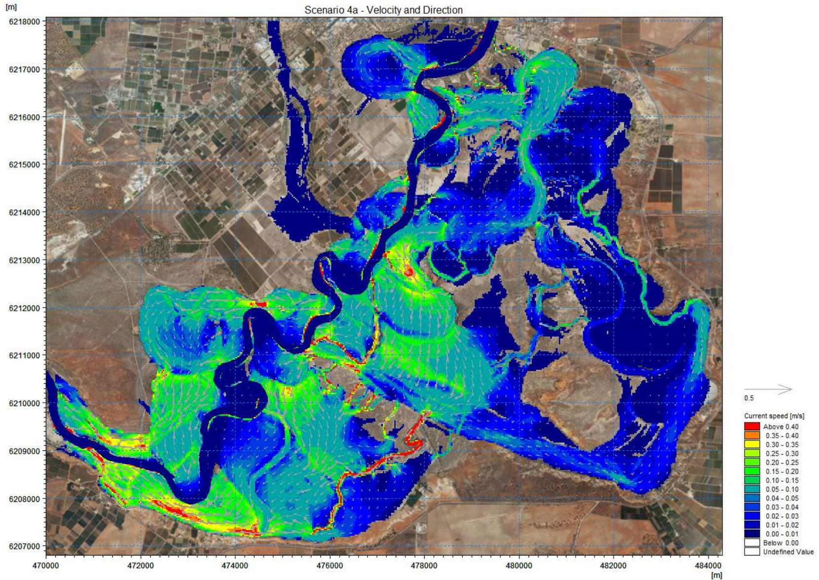
**Figure 6.1 Velocity distribution and direction for River Murray flow of 90 000 ML/d with all structures open. Environmental regulators at Tanyaca and Pike at 100% of concept design size**
