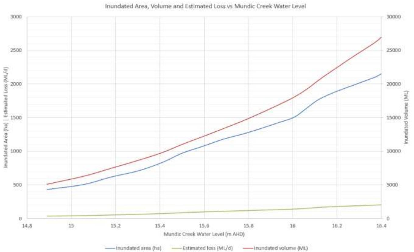
**Figure 7.7 Inundated area (ha), impounded volume (ML) and estimated loss (ML/d) versus Mundic Creek water level**
