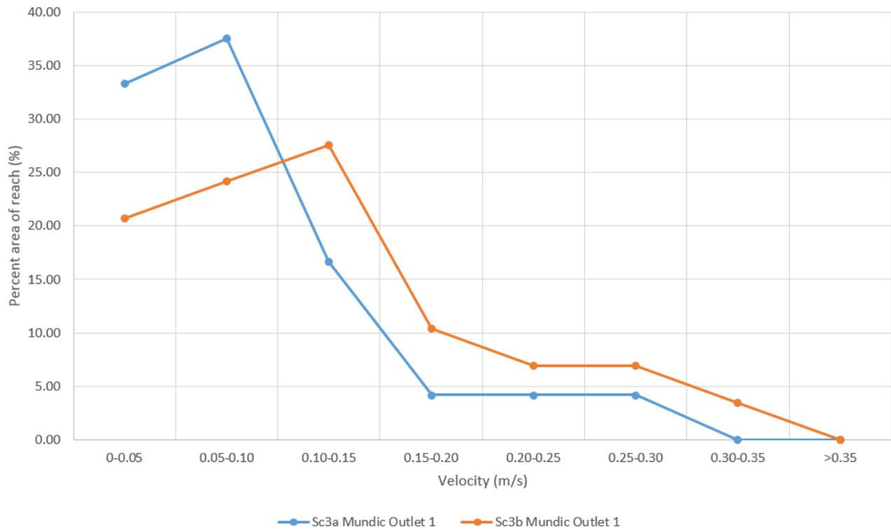
**Figure 5.5** Velocity distribution by percent of reach in Mundic Creek Northern Outlet for Scenario 3 simulations (refer to Figure 2.1 for location)
