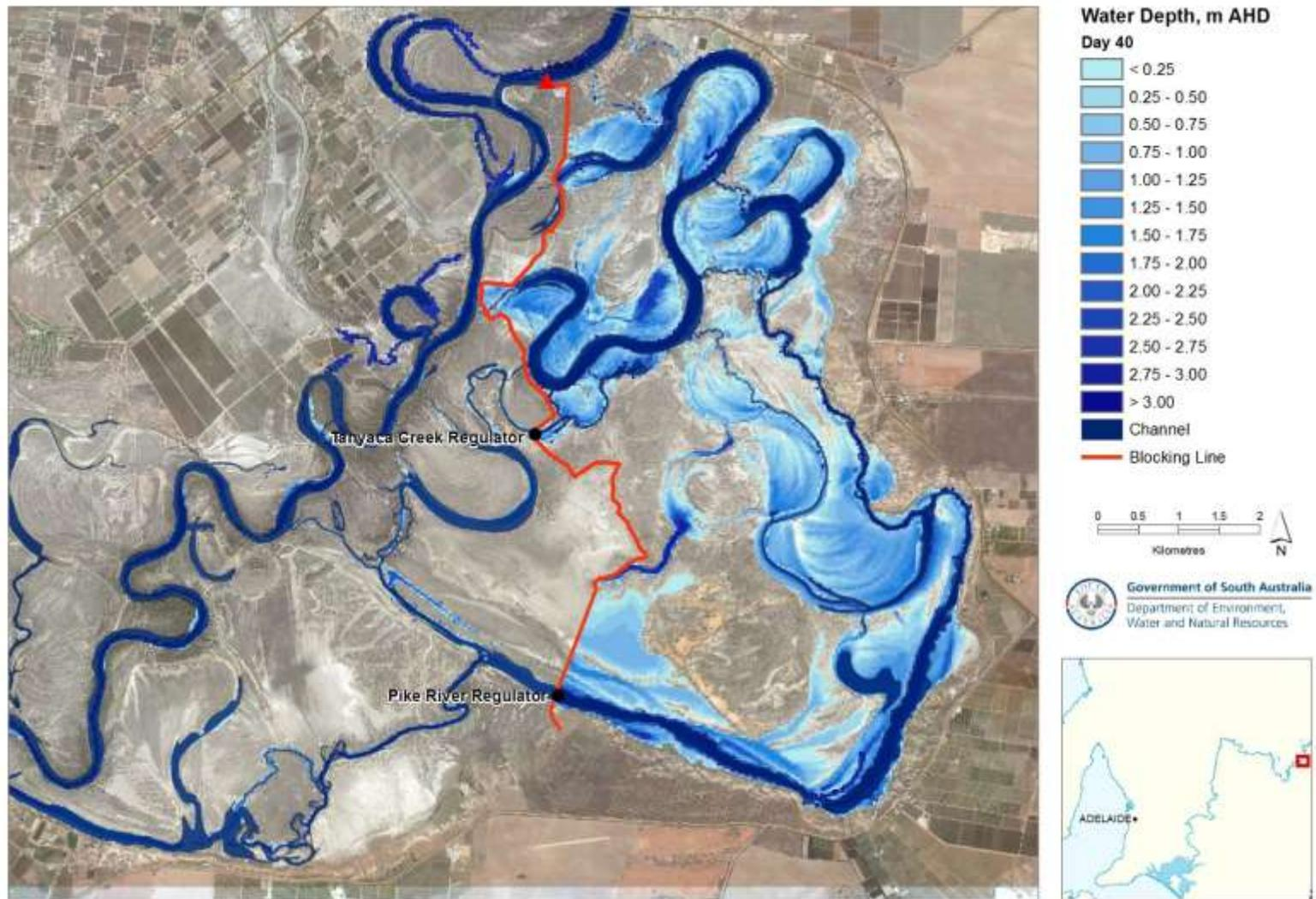
**Figure 9.7 Inundation extent and water depth at Day 40 (water level at Pike Regulator 16.40 m AHD) of managed inundation under Alternative 2 blocking alignment**
