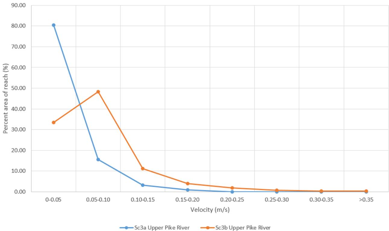
**Figure 5.11 Velocity distribution by percent of reach in Pike River (upstream of Rumpagunyah junction) for Scenario 3 simulations (refer to Figure 2.1 for location)**
