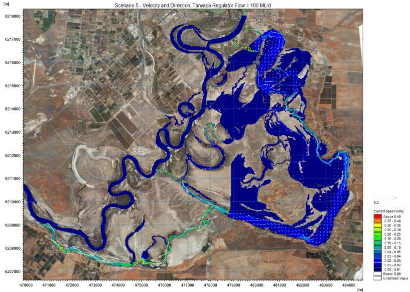
**Figure 7.4 Velocity distribution and flow direction at an inundation level of 16.4 m AHD with alternative Pike River environmental regulator placement and a flow of 100 ML/d through Tanyaca Creek**
