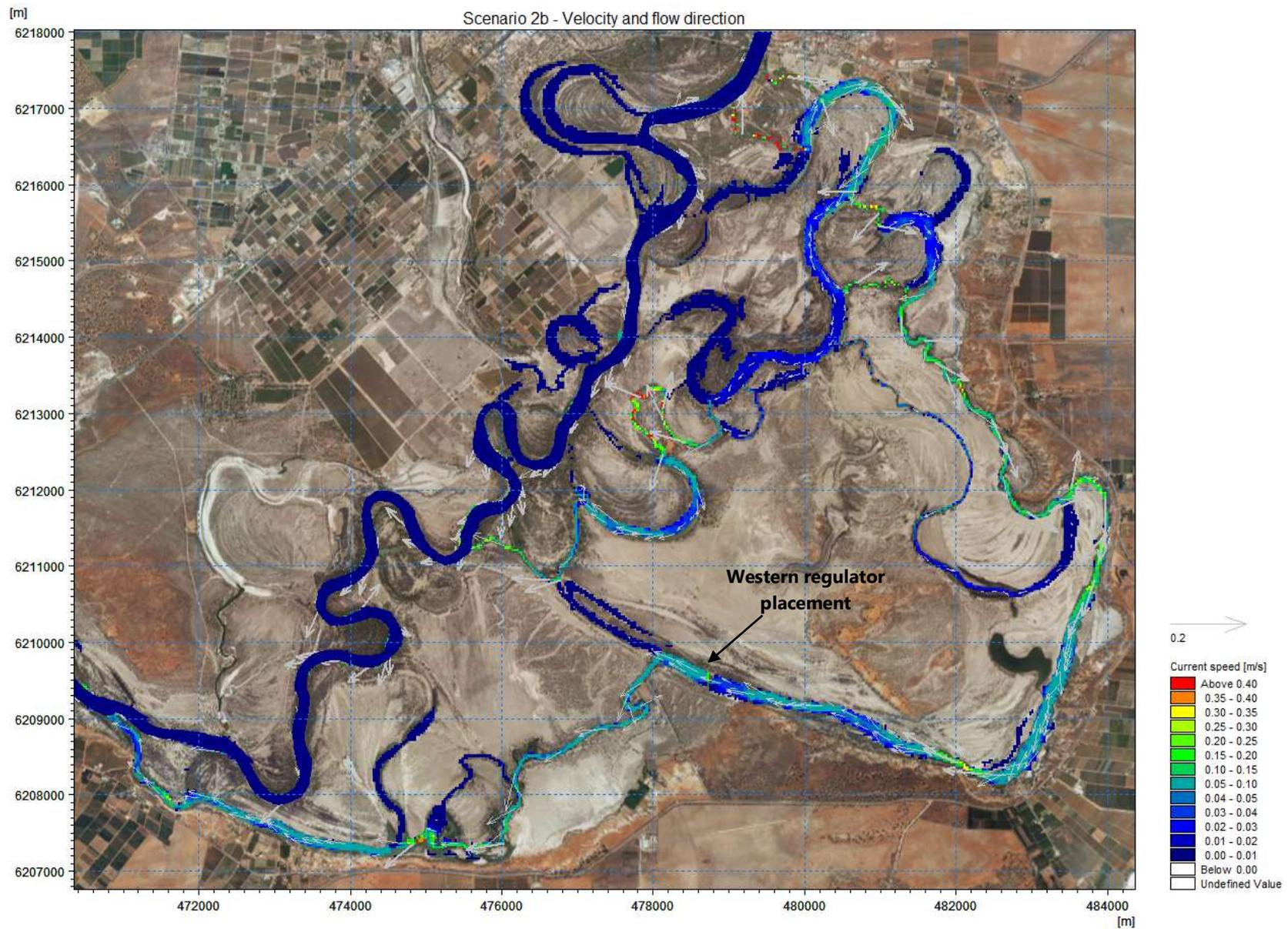
**Figure 4.4 Velocity and flow direction for an inflow of 1200 ML/d and Tanyaca flow of 400 ML/d (Scenario 2b)**
