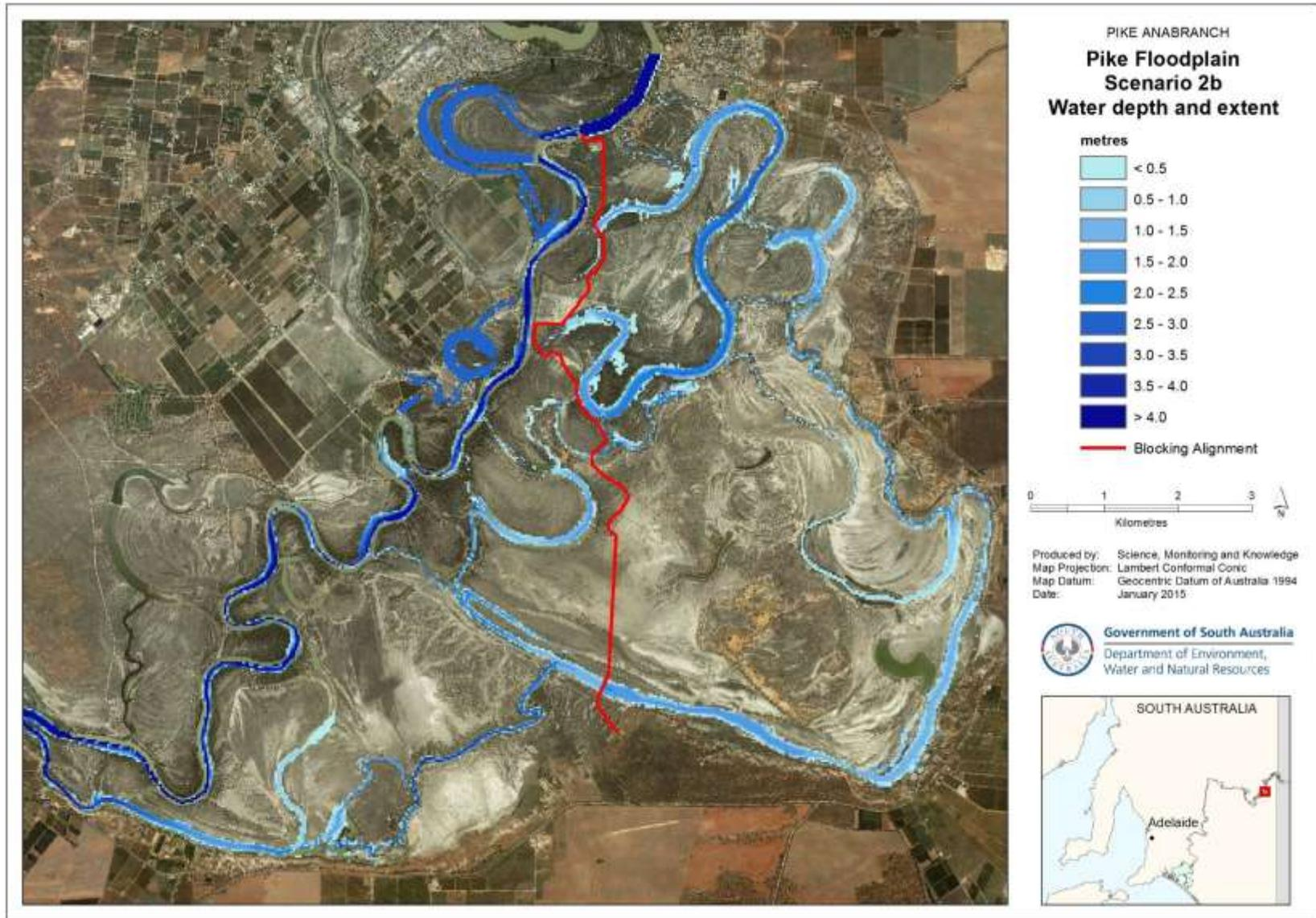
**Figure 4.3 Water depth and extent for an inflow of 1200 ML/d and Tanyaca flow of 400 ML/d (Scenario 2b)**
