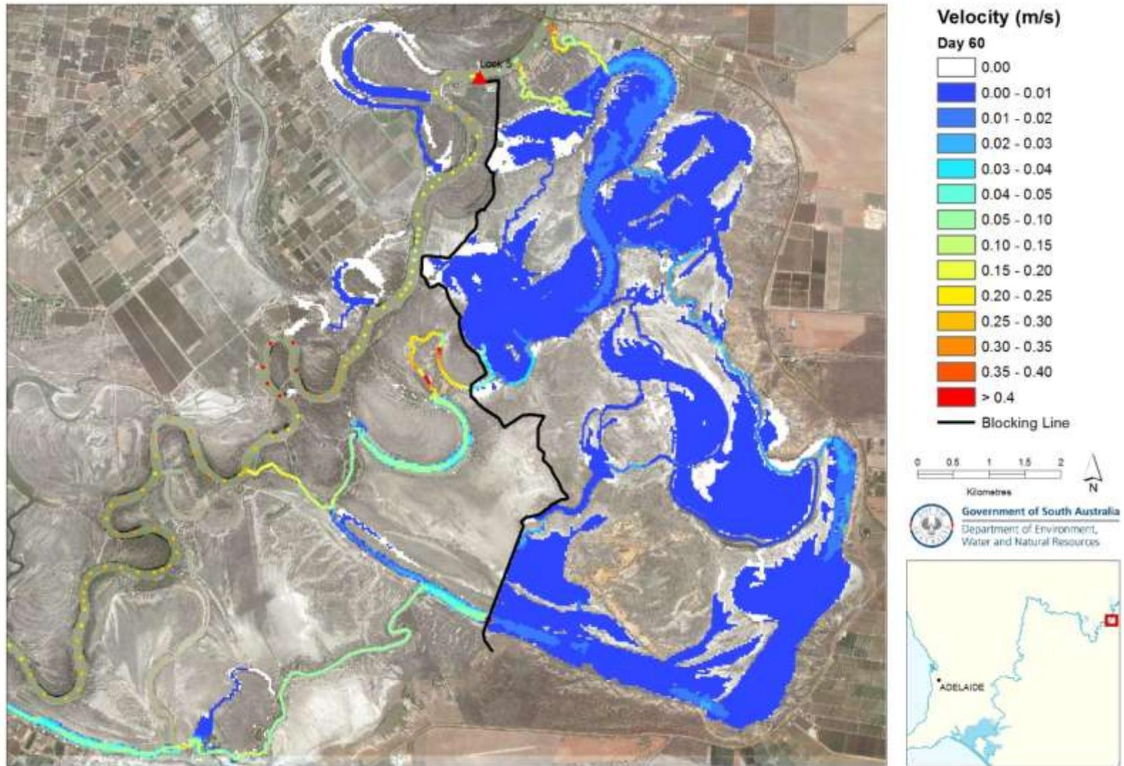
**Figure 9.19 Velocity distribution at Day 60 (water level at Pike Regulator 16.34 m AHD) of managed inundation under Alternative 2 blocking alignment**
