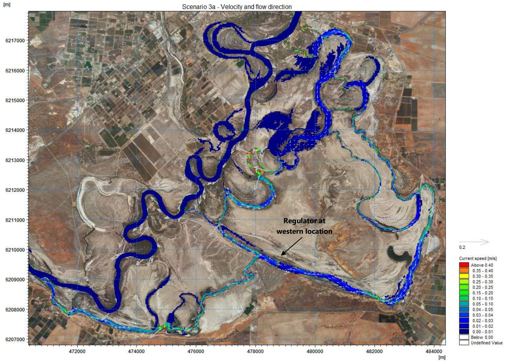
**Figure 5.2 Velocity and flow direction for an inflow of 800 ML/d and minor regulators on Mundic Creek outlets passing 400 ML/d (Scenario 3a)**
