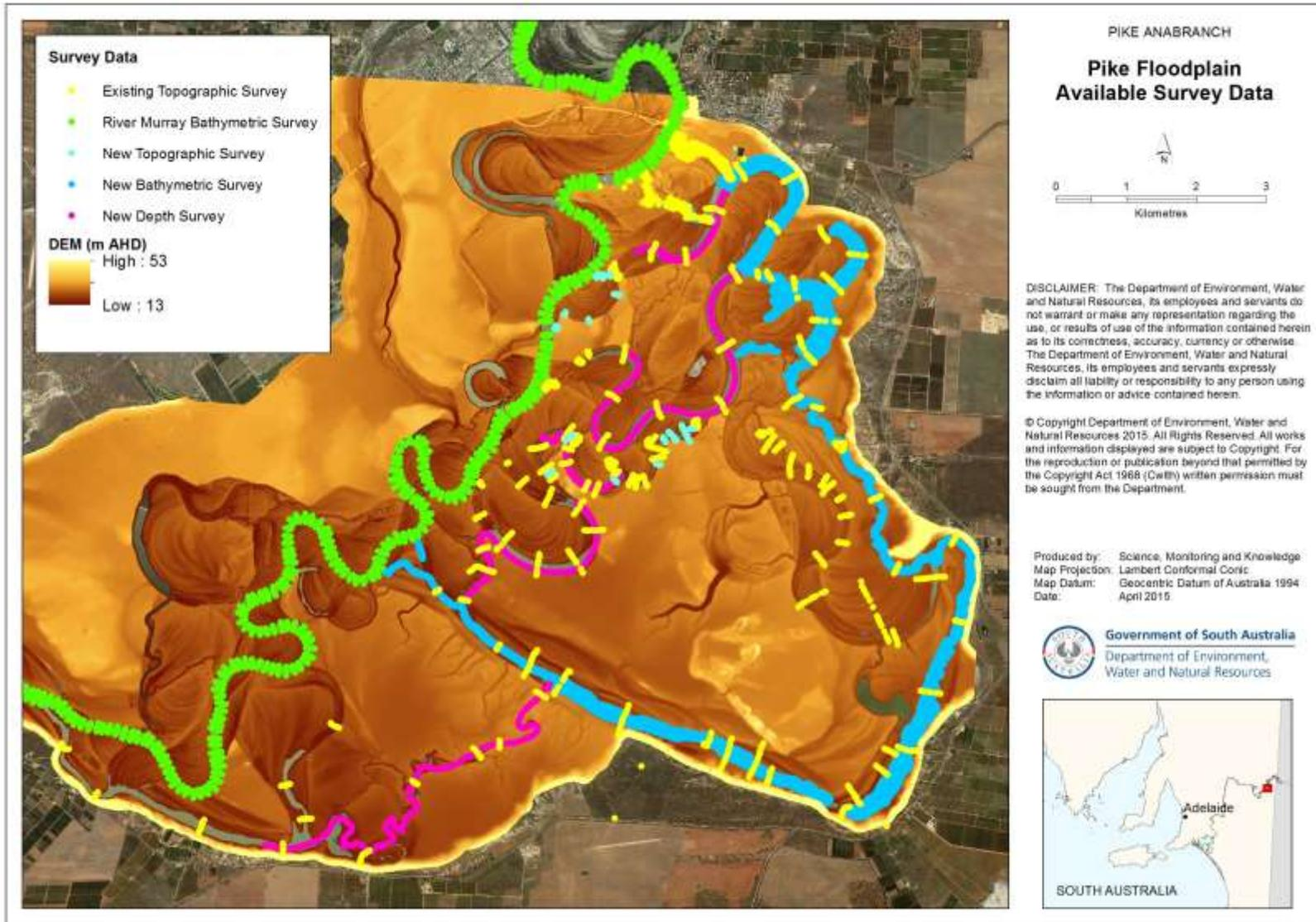
**Figure 2.2 Topographic and bathymetric survey data for Pike Floodplain**
