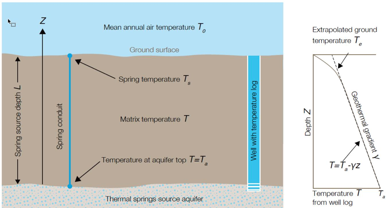
**Figure 3.12. Schematic showing modelled thermal spring source depth (Wolaver *et al.*, 2013)**
