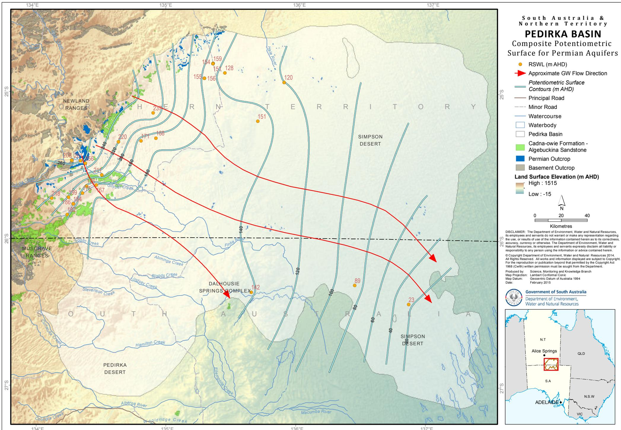
**Figure 3.4. Time composite potentiometric surface of Permian aquifers of the Pedirka Basin (Wohling et al., 2013b)**
