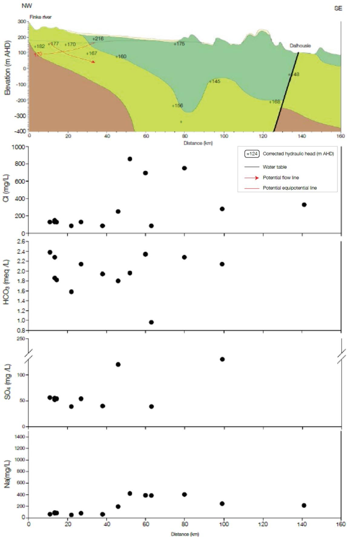
**Figure 3.10. Schematic geological cross-section from Finke River to Dalhousie Springs and groundwater concentrations of chloride, alkalinity, sulfate and sodium (Priestley *et al.*, 2013)**
