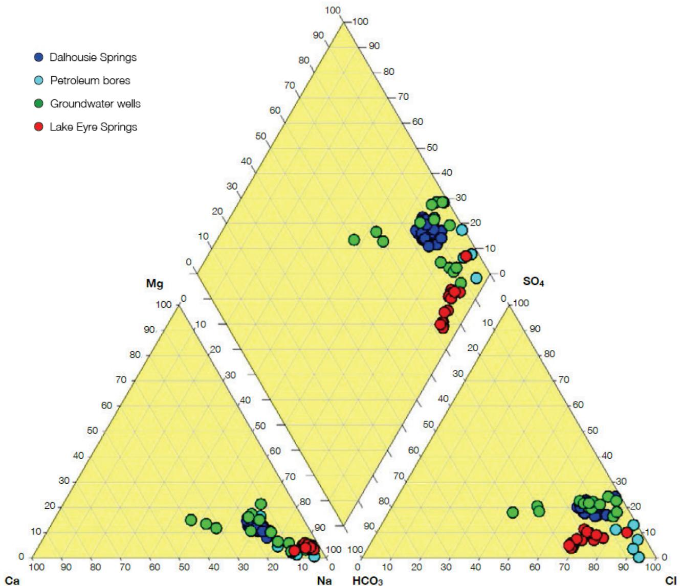
**Figure 3.8. Hydrochemical signatures of Dalhousie Springs complex discharge, groundwater and Lake Eyre Springs (Wolaver *et al.*, 2013)**
