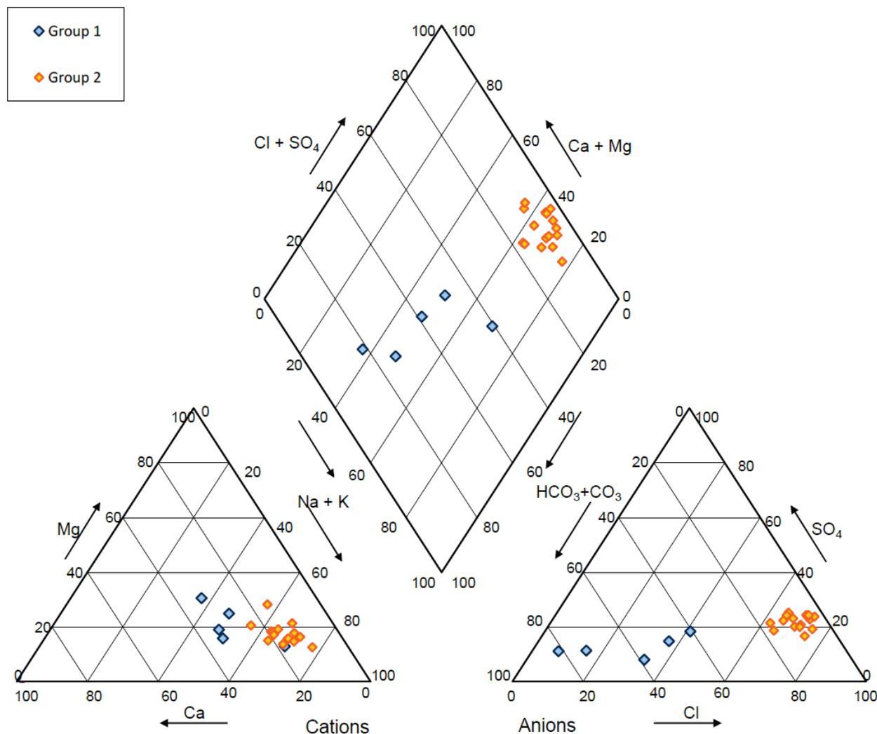
**Figure 3.9. Piper plot of Permian Crown Point formation groundwater samples showing two distinct groupings (Wohling *et al.*, 2013b)**
