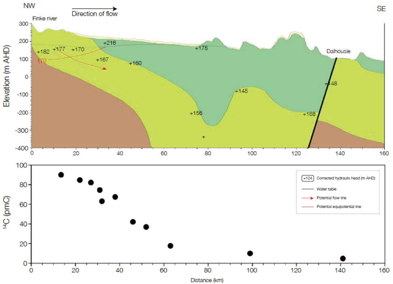
**Figure 3.11. Schematic geological cross-section from Finke River to Dalhousie Springs and groundwater concentrations of  $^{14}\text{C}$  (percent modern carbon) (Priestley *et al.*, 2013)**
